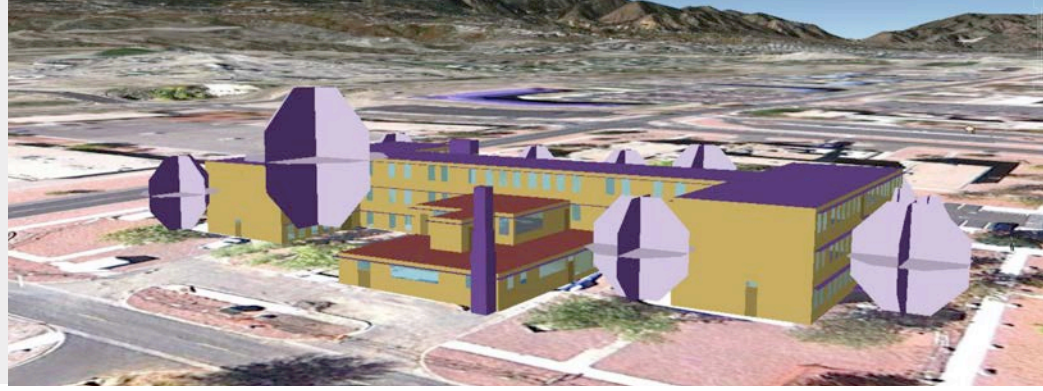
Figure 21. Final Building 1219 energy model with PV and shading objects Image Credit: © 2013 Google Earth, alterations by Matthew Leach, NREL.
