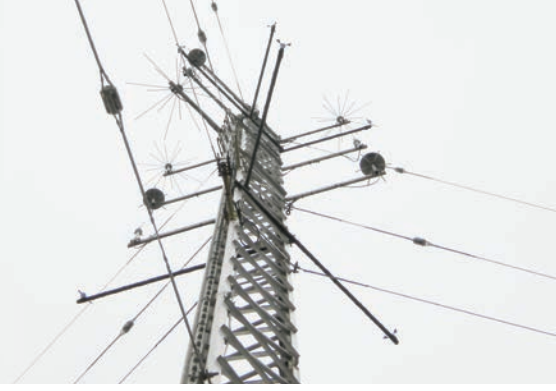
Figure 39. Meteorological tower instrumented with anemometry Photo by Dan Olis, NREL
