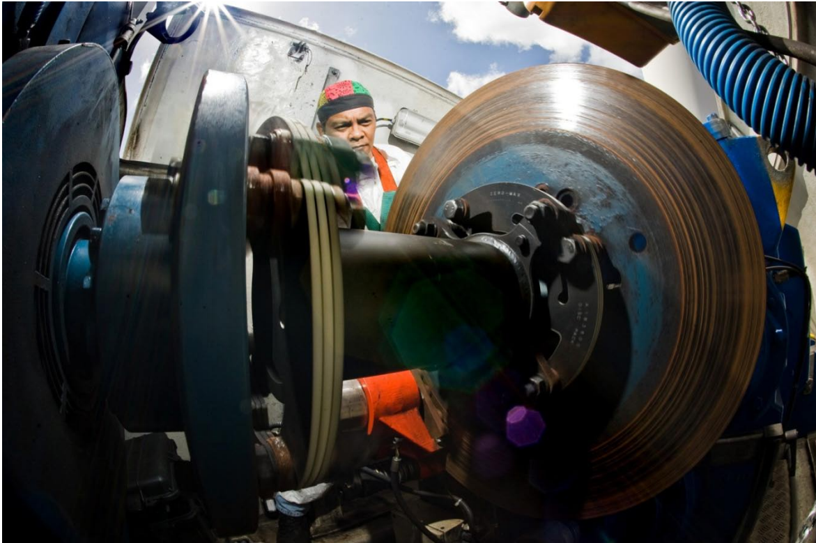
Figure 109. A brake disk on a 900 kW wind turbine at Ascension Auxiliary Airfield. 213
