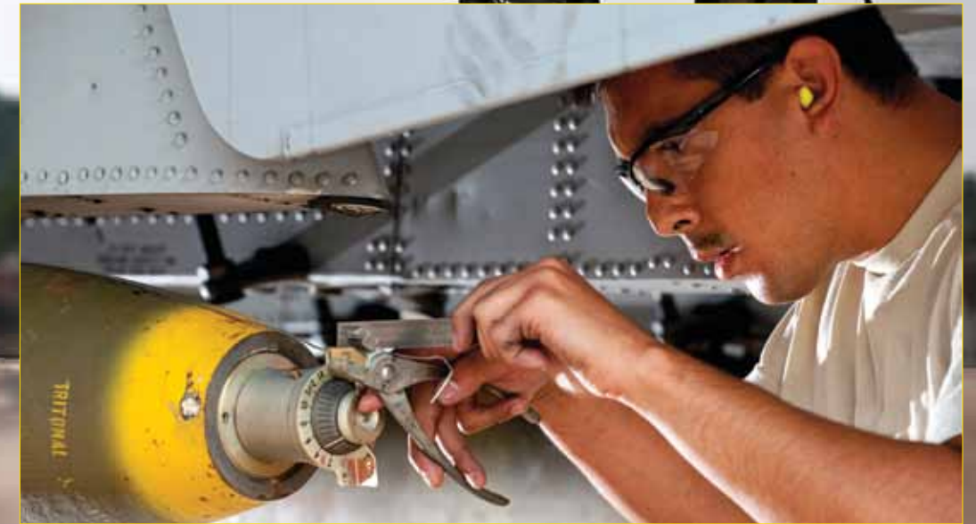
Senior Airman Cruz Galvan, a member of the 122nd Weapons Load shop, cuts the arming wire on a bomb.
