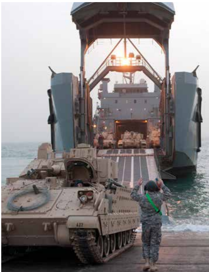
Army vehicles are loaded onto Army Reserve Logistics Support Vessel-8 Major General Robert Smalls at Kuwait Naval Base, using a ramp that extends through the open bow of the ship.
