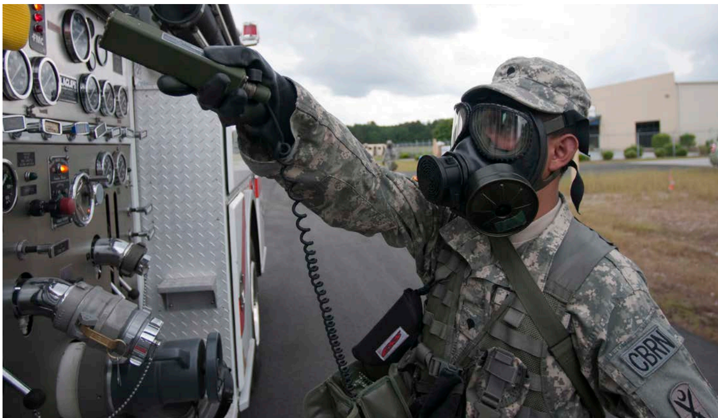
SPC Maung Koko, with the 108th Chemical Company from South Carolina Army National Guard, used radiation detection equipment to find harmful gamma and beta radiation on contaminated vehicles during an Ardent Sentry exercise held in Ridgeland, South Carolina. A simulated contaminated convoy is processed by the 108th Decontamination Platoon before being allowed entry to the point of distribution to pick up food and water supplies needed for civilians after a natural disaster. (Photo by SSgt Jorge Intrigo, U.S. Air National Guard)
