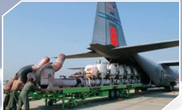
Airmen from the North Carolina Air National Guard's 145th Airlift Wing push a modular airborne fire fighting system onto a C-130 Hercules. The system is a series of pressurized tanks that hold 3,000 gallons of flame-retardant liquid. The retardant is dropped along the leading edge of a fire to block the spread of flames.
