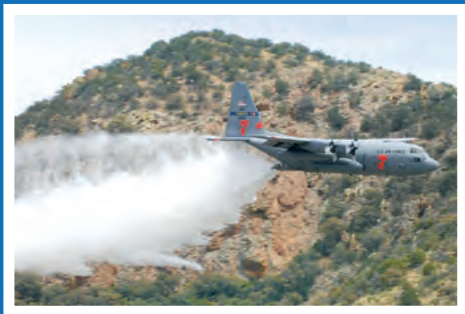
The Modular Airborne Firefighting System (MAFFS) is an important and effective tool used to fight wildfires nationwide and is placed onboard C-130 Hercules aircraft as shown here.
