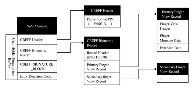
Figure 7. Card Holder Fingerprints Container Structure
