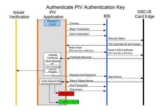
Figure 8. Authenticate PIV Authentication Key Sequence diagram
