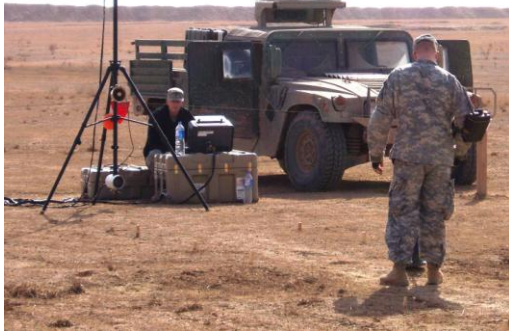
Sweep Monitoring System shown with tripod, with tracking cameras mounted top and bottom, cabled to instructor's base station computer.
