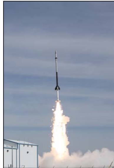
A Terrier Black Brant sounding rocket is launched in support of a NASA mission to collect data on the sun. The data was then used to calibrate several solar observations satellites. Courtesy Photo
