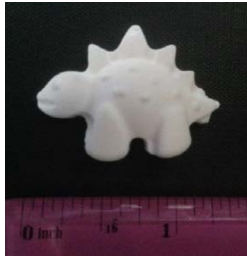
Fig. 9 Complex-shaped cast green body using the ISOBAM gelling system and slurry preparation procedure outlined in Section 2.2
