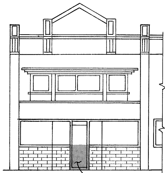
TEMPORARY DOORWAY FLOOD SHIELD SEATED AGAINST RUBBER GASKET.
