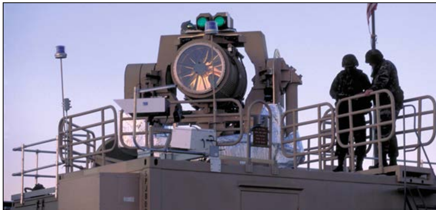
This beam director was used for the Mobile Tactical High Energy Laser and has been reformatted to support the Solid State Laser Testbed Experiment at High Energy Laser Systems Test Facility at White Sands Missile Range, NM. (U.S. Army photo)
