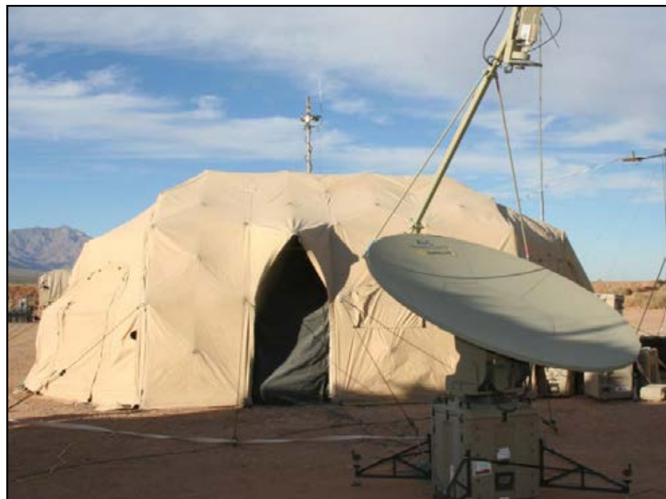
The Army's next generation high-bandwidth Secure Internet Protocol Router/Non-secure Internet Protocol Router Access Point, or SNAP, ground satellite terminals will include military satellite and secure Colorless Core capability. The SNAP shown here was part of NIE 13.1 at WSMR. (Photo: A. Walker)
