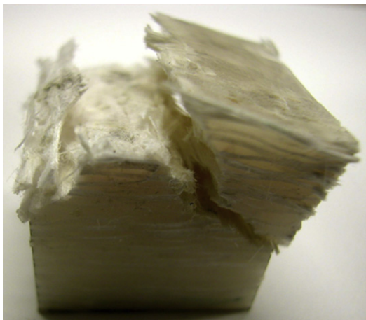
Fig. 8. Typical damage surface of a fractured specimen.
