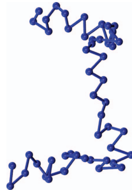
FIG. 9. Example structure of an mSRP chain without an angle potential ( N = 50 , b = 100 , d_c = 0.9 ).
