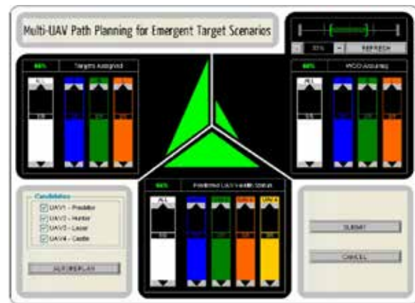
Fig. 4. Supervisory control of four UAVs—configural display is the center panel with three green triangles indicating the costs of planned operations (image adapted from [111], with permission).
