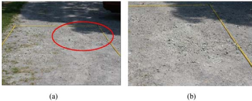
Fig. 3. Photograph of DE region May 22, 2008 test conducted at U.S. Army Research Laboratory, Adelphi, MD site. 3(a) DE test-bed (red oval area represents buried target and 3(b) a close up of the DE region (clay-gravel-soil mixture).
