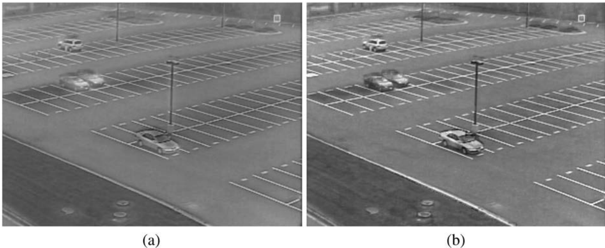
Fig. 6 Fusion by selecting the maximum coefficient of the gradient pyramids (a) and morphological pyramids (b).
