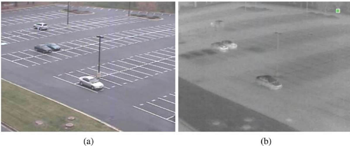
Fig. 1 Example of a color visible (a) and an LWIR (b) image in the FPSS dataset.
