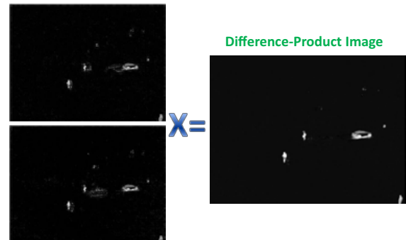
Fig. 9 Enhancement of target signatures and suppression of trailing effects and noises via a DPI.
