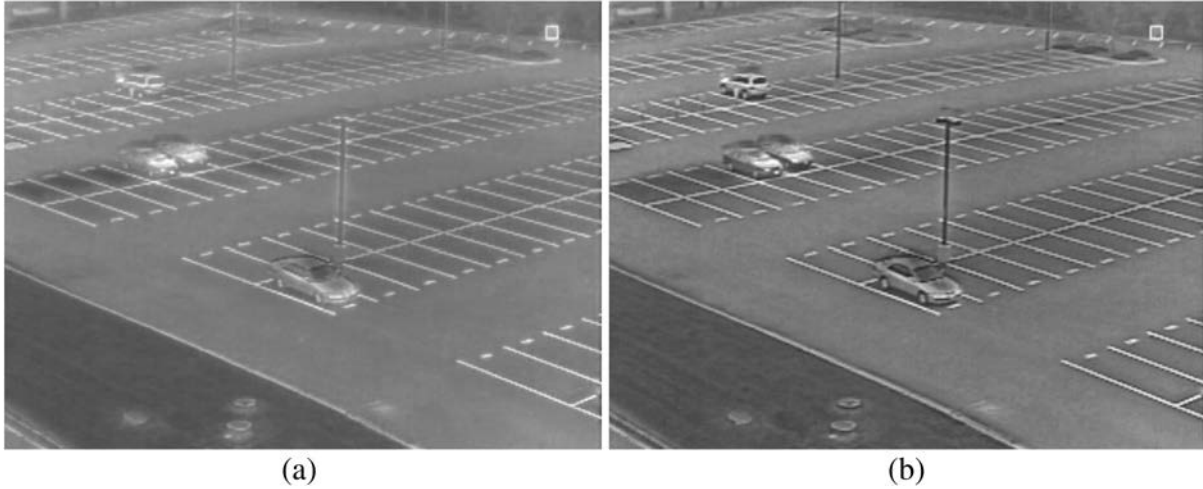
Fig. 5 Fusion by selecting the maximum coefficient of the ROLP pyramids (a) and contrast pyramids (b).
