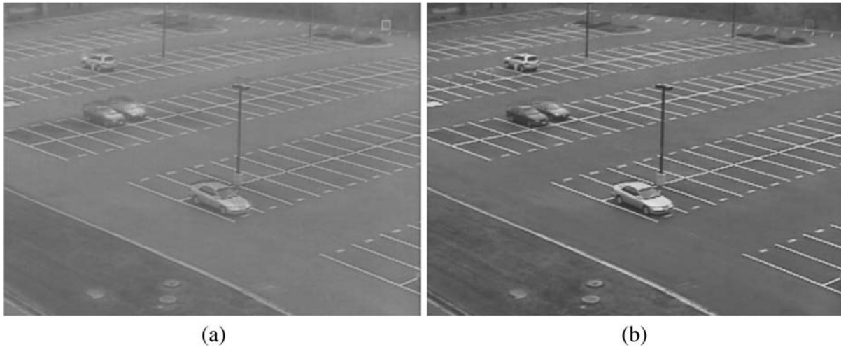
Fig. 2 Fused image through simple average (a) and PCA-weighted average (b).
