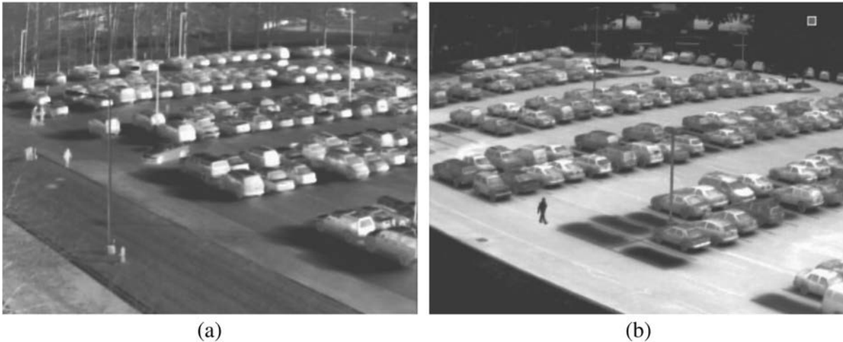
Fig. 10 Human LWIR signatures reverse polarity in winter (a) and summer (b).
