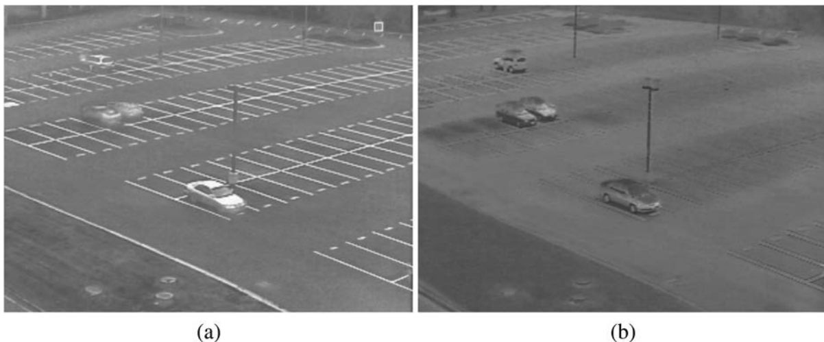
Fig. 3 Fusion by selecting maximum (a) and minimum (b) pixel intensities.
