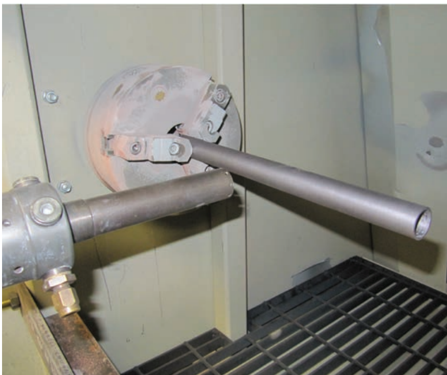
Cold spray consolidation of a tantalum tube.
