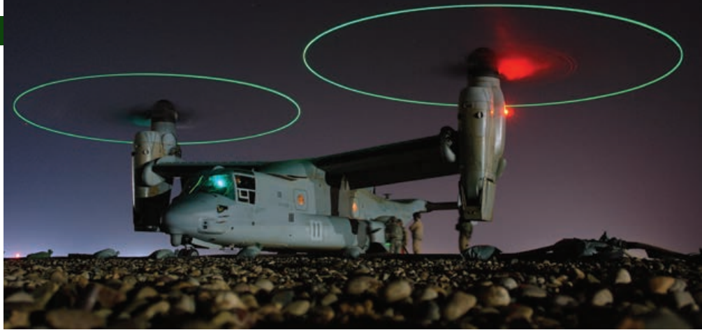
The V-22 Osprey is a multi-mission, military tiltrotor aircraft capable of vertical take-off and landing (VTOL).
