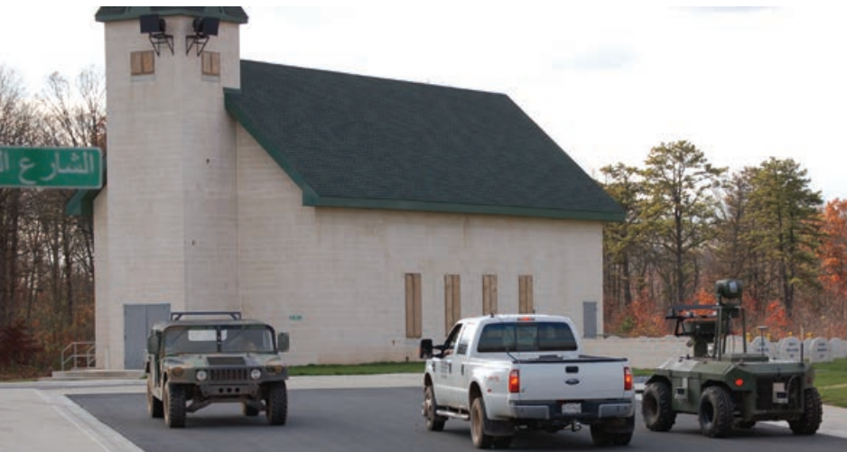
Autonomous detection, tracking, and avoidance of vehicular traffic by a UGV in an urban environment during a portion of the Robotics CTA capstone experiment at Fort Indiantown Gap, Pa.
