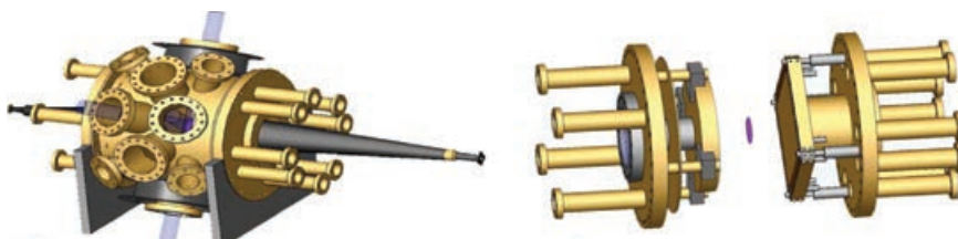
Schematic of the ultra-high vacuum magneto-optical trap (MOT) chamber used for the successful laser-cooling of molecules: the schematic illustrates (a) the full chamber geometry, including MOT coils and laser beams, as well as feeds for inserting and detecting microwave power in the cavity, and (b) a view of the interior of the chamber, showing the cavity geometry and various mounting fixtures. The potential trap volume is illustrated by the purple ellipsoid at the center of the panel. [Image credit: David DeMille]
