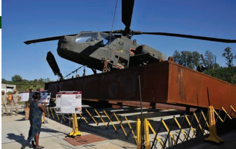
An AH-64D Apache attack helicopter is mounted to the ARL Rotorcraft Survivability and Assessment Facility’s tilt-table for later live-fire and other tests and evaluations. The new RSAF facility tests U.S. military and foreign rotor aircraft to help keep Warfighters safe from threats.
