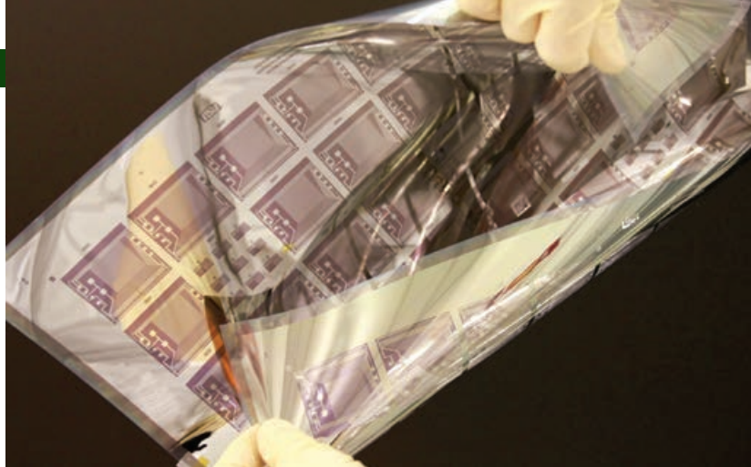
A generation II sized panel of displays in plastic fabricated at the Flexible Display Center.
