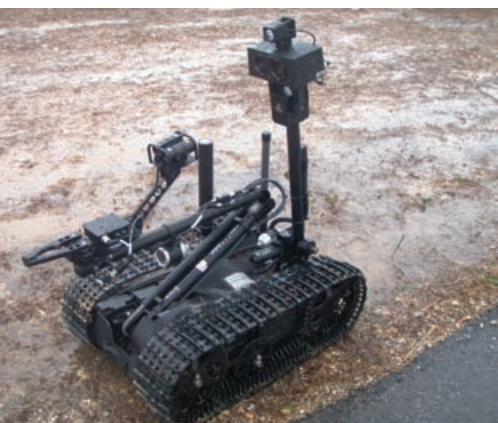
TALON robot system equipped with 3-D cameras on the arm and rear mast.
