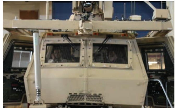
Spinel based transparent armor on FMTV 1083A1 P2 for TARDEC/ARL TWVS ATO demonstrator undergoing testing.
