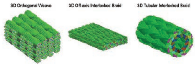
Figure 1: 3-D Fabric Fiber Architectures Generated by Using the Textile Process Simulation Code.
