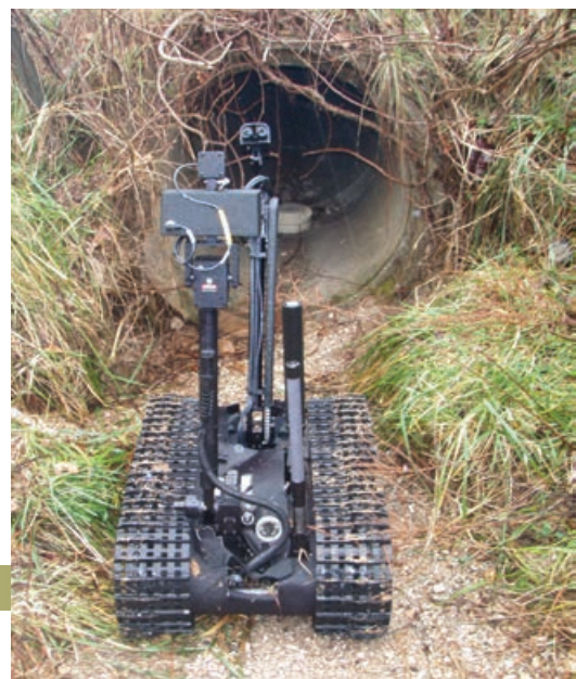
TALON robot preparing to investigate for potential threats in a road culvert.
