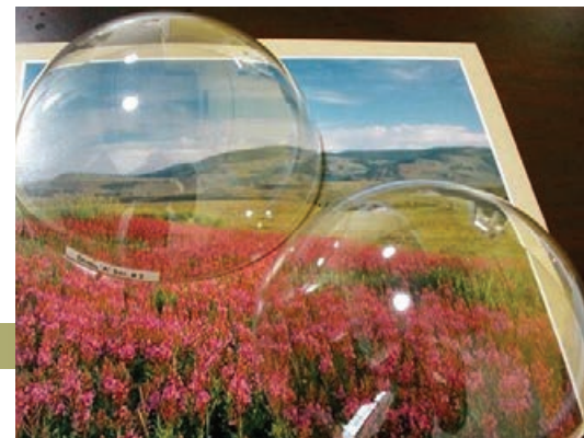
Sintered spinel domes for Joint Air to Ground Munitions (JAGM) Army/Navy, and small diameter bomb dome Air Force.
