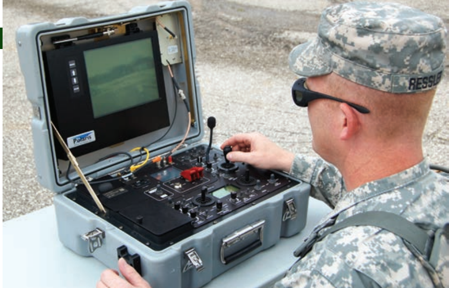
Soldier operating a TALON robot on a simulated mission using the fully integrated 3-D display.
