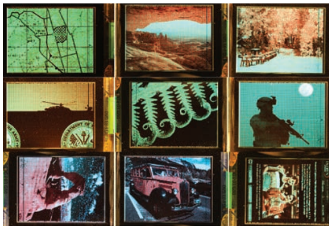
An array of flexible Color Emissive Displays developed at the Flexible Display Center. ARL contributed to the process development.
