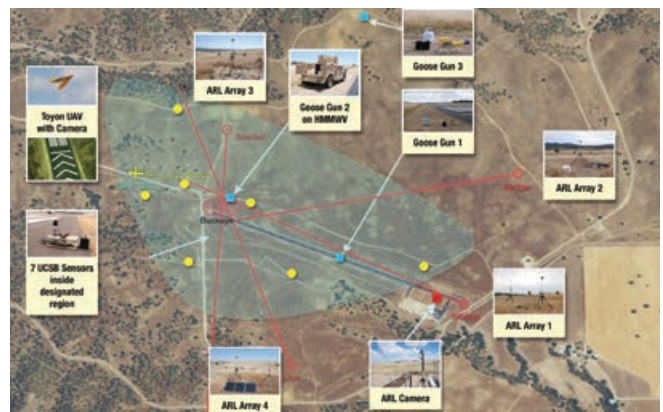
Persistent ISR scenario with networking and interoperability of two coalition networks: one sensor network with four acoustic arrays plus one fixed mounted camera and a second sensor network with seven low-cost unattended ground sensor (UGS) plus one unmanned aerial sensor (UAS) with visual camera onboard plus one UAS data harvester.
