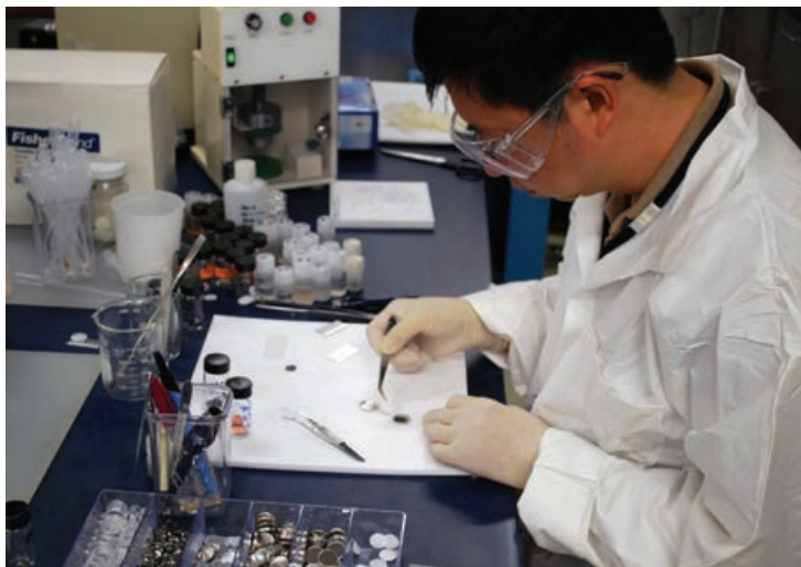
Dr. Kang Xu assembling a test cell that uses a high voltage electrode and electrolyte.
