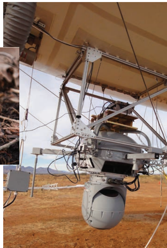
Imager gondola on the Persistent Ground Surveillance System aerostat.
