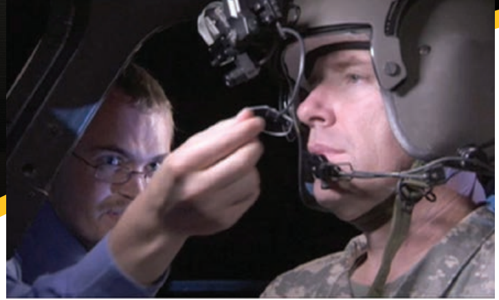
ARL researcher fitting an Army aviator with an eye tracker.
