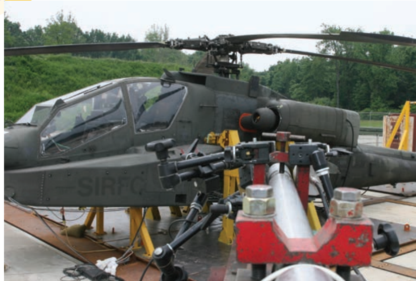
Apache Block III Improved Drive System test setup, gun view.
