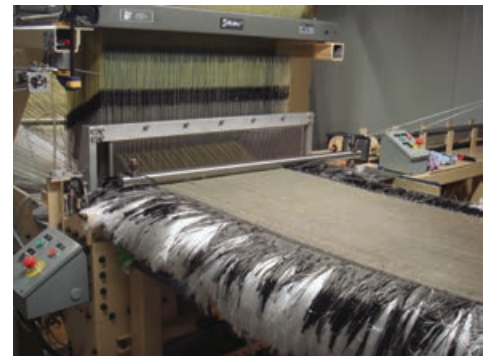
A Jacquard loom weaving a 3-D reinforced glass, carbon, and aramid fiber hybrid architecture.
