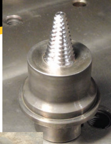
Typical friction stir welding tool used for aluminum alloy plates.
