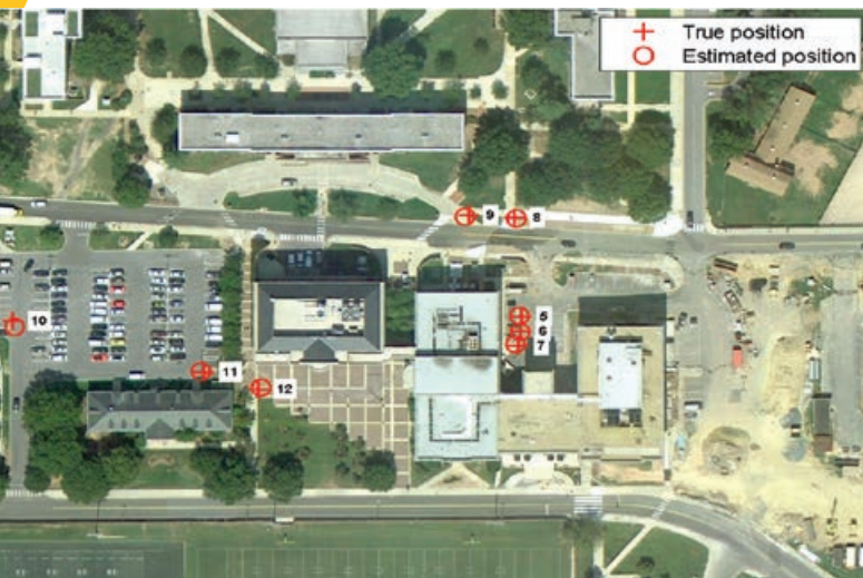
ARL has developed algorithms that can localize the robot in an urban environment to within 1 meter without a global positioning system (GPS) and without visiting the site in advance.
