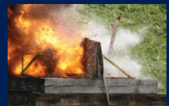
Ballistic vulnerability test of a static helicopter main rotor blade.
