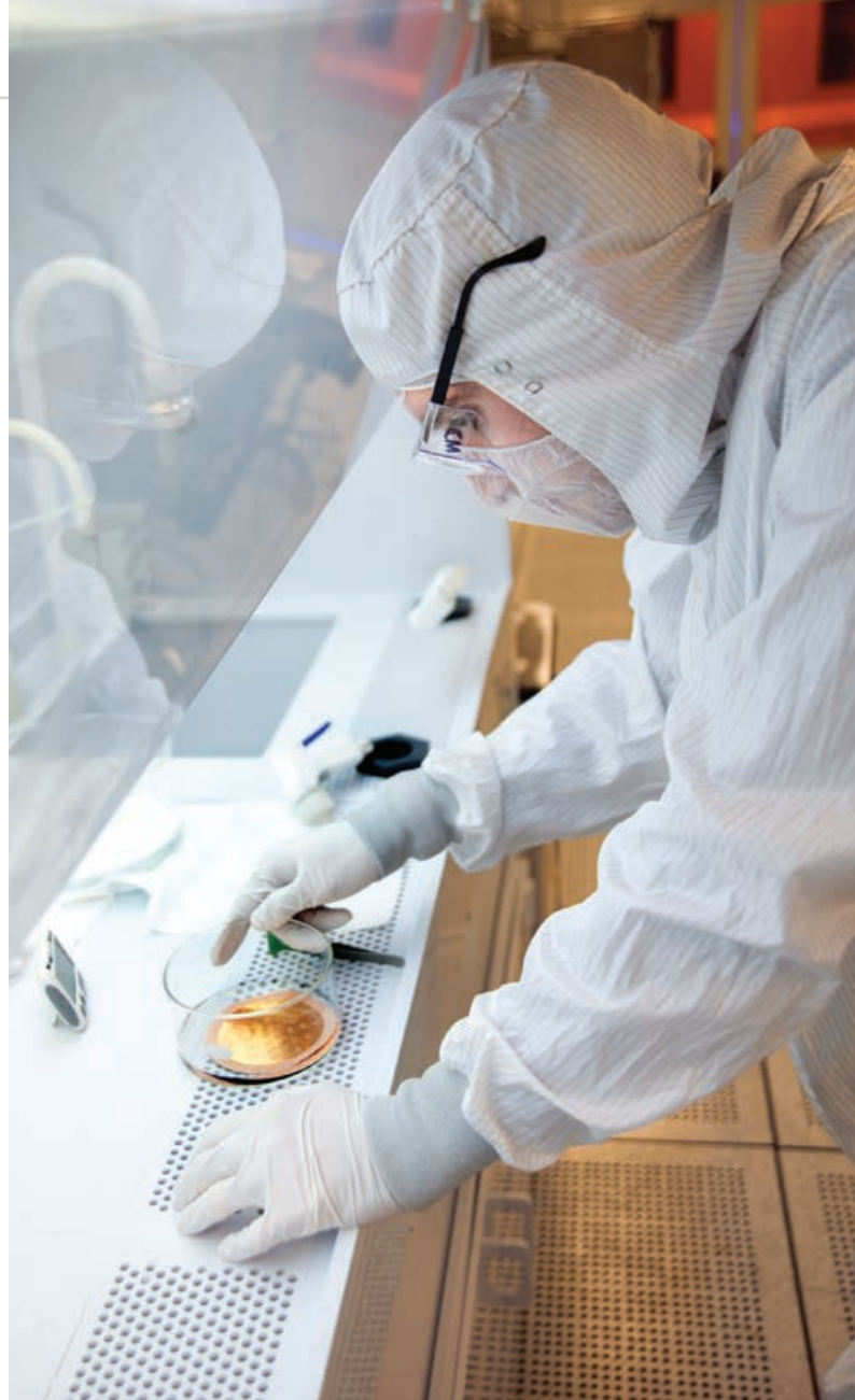
Dr. Chris Meyer processes a silicon wafer in the ARL cleanroom to test fabrication methods for realizing high density, efficient power microinductors.
