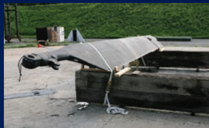
Ballistic vulnerability test of a static helicopter main rotor blade.
