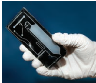
Disposable microfluidic cartridge enables rapid isolation of synthetic recognition reagents used for sensing biological threats.
