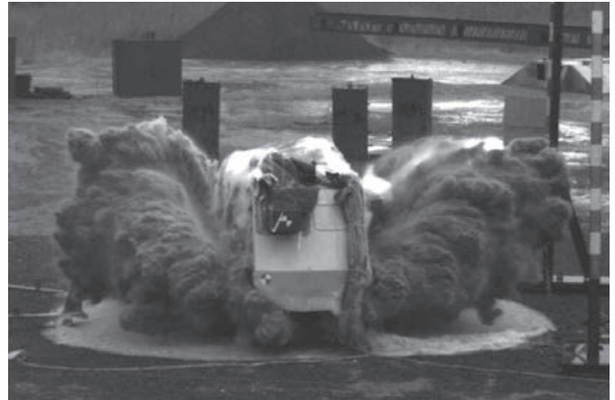
High speed video capture of underbody blast test using a generic hull to demonstrate the under-body blast environment to medical researchers.
