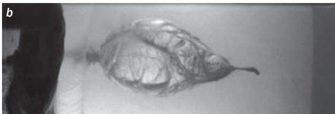
High-speed images in gelatin block behind ceramic armor of interest: (a) for conventional state-of-the-art 5.56mm armor piercing impact (no perforation), (b) for 5.56mm advanced armor piercing technology round impact.
