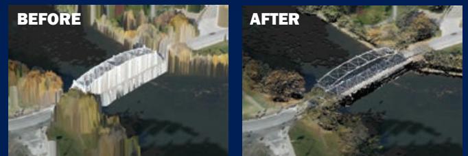
Before and after images of a bridge, where the point cloud is draped to improve visualization for the user.
