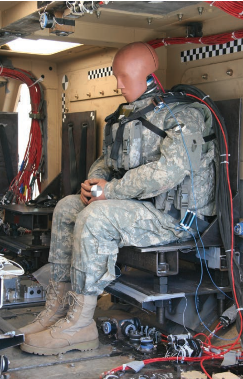
High speed video capture of underbody blast test using a generic hull to demonstrate the under-body blast environment to medical researchers.
