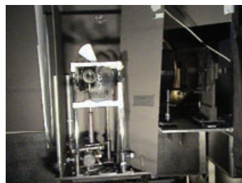
Eye optical cross-section (OCS) study subject location on Fourier Transform Range Simulator (FTRS) table showing pupil adjustment source and chin rest.
