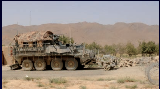
Improved Stryker Infantry Carrier Vehicle, one of the seven DVH configurations analyzed.
