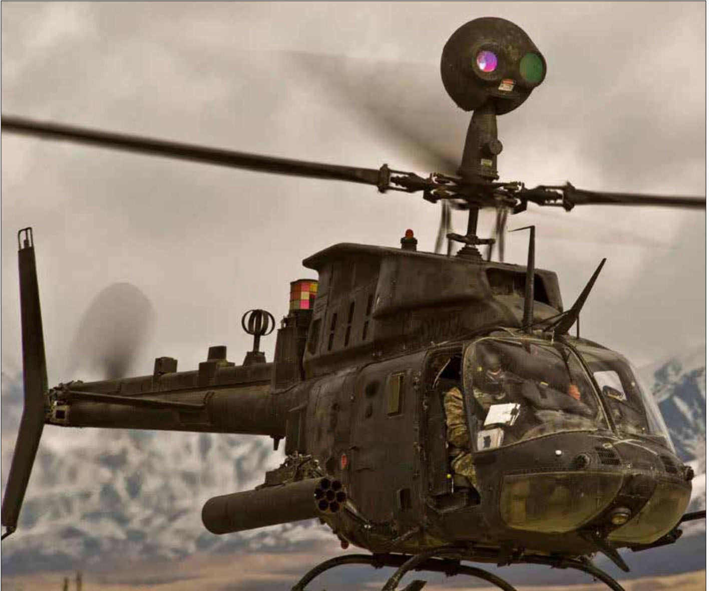
A Bell OH-58 Kiowa, a single engine, single rotor helicopter used for observation, utility and direct for support. U.S. Army photo released..
