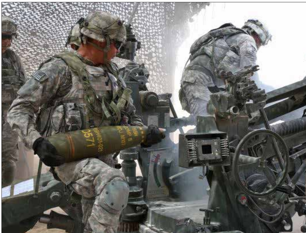
A soldier assigned to A Battery, 2nd Battalion, 12th Field Artillery Regiment, 1st Stryker Brigade Combat Team, 4th Infantry Division, loads M107, 155mm projectile ammunition for an M777 Light Towed Howitzer during calibration for Decisive Action Rotation 15-10 at the National Training Center, Sept. 10, 2015. (Photo: Army/Spc. Ashley Marble)
