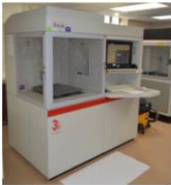
Figure 3 Stereolithography machines (SLA) are the workhorse of 3DMAC; they can produce large models often used by orthopedics for pre-surgical planning
