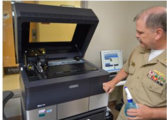
Figure 2 A materials jetting technique machine produces plastic models for dental implants and surgical guides
