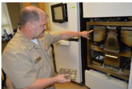
Figure 4 The electron beam melting process is used to fabricate titanium implants and prosthetic parts
