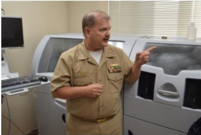
Figure 1 Powder binding printers produce color pre-surgical models often used in neurosurgery to show vessels and tumors
