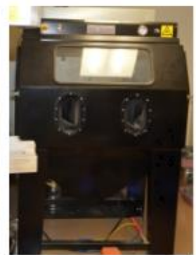
Figure 6 A larger recovery system allow for recycling of titanium powder
