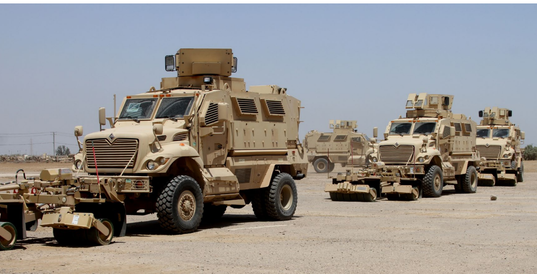
The ISF receives a shipment of 30 MaxxPro mine-resistant, ambush-protected (MRAP) vehicles with mine-roller attachments at Camp Taji, Iraq, July 13, 2015.
