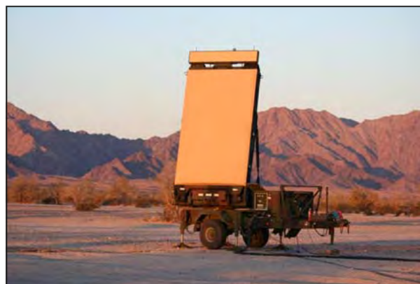
A Ground/Air Task Oriented Radar (G/ATOR) undergoes development testing during an exercise at Marine Corps Air Station Yuma. Courtesy of G/ATOR Program Office (photo by USMC)
