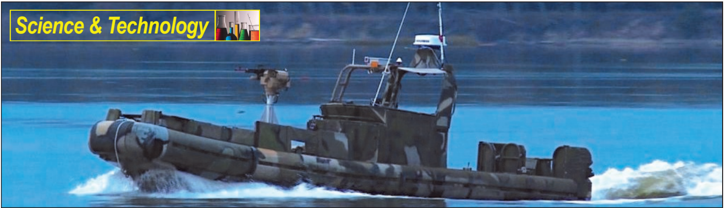
An autonomous unmanned surface vehicle (USV) transmits real-time targeting data to an Aegis weapon system that engaged a target on the Potomac River Test Range with the MK34 5 inch/62 caliber gun weapon system during a surface warfare integration test. U.S. Navy photo by Patrick Dunn
