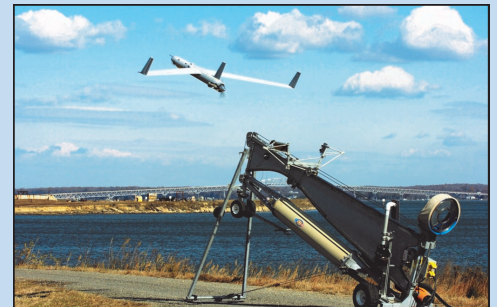
A Scan Eagle unmanned aerial vehicle (UAV) launches from the Naval Surface Warfare Center Dahlgren Division (NSWCDD) Potomac River Test Range. NSWCDD scientists and engineers demonstrated how the science of integration makes surface warfare systems interoperable with unmanned systems during a surface warfare integration experiment. U.S. Navy photo by John Williams.
