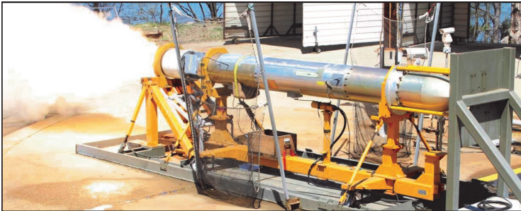
Video screen capture from a Tactical Tomahawk missile Functional Ground Test at Naval Surface Warfare Center Indian Head Explosive Ordnance Disposal Technology Division's (NSWC IHEODTD) Large Motor Test facility in Indian Head, Md. High-speed cameras document the missile's progress throughout the event. U.S. Navy photo.
