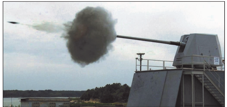
An MK45 5-inch lightweight gun fires on a fictitious threat on the Potomac River Test Range during a surface warfare integration test Sept. 29. Naval Surface Warfare Center Dahlgren Division (NSWCDD) engineers relied on unmanned surface and air vehicles to guide live gun fire onto distant targets, demonstrating a new integrated surface warfare capability in a maritime environment. U.S. Navy photo by Patrick Dunn.
