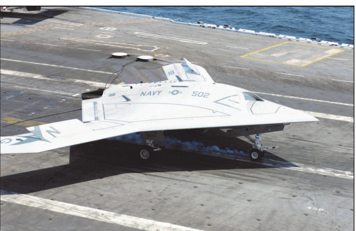
NORFOLK, Virginia (July 10, 2013) — The U.S. Navy demonstrated the first X-47B Unmanned Combat Air System (UCAS) carrier-based arrested landing on board USS George H.W. Bush (CVN 77) off the coast of Virginia. The successful landing marks the first time a tailless, unmanned autonomous aircraft landed on a modern aircraft carrier. Photo by Captain Jane E. Campbell
