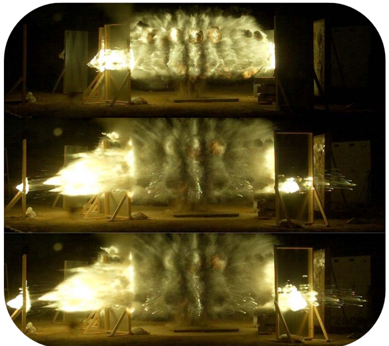
High speed video images capture the formation and launch of HDRM fragments from the detonation of a cylinder of HDRM filled with C4 explosive. The explosively formed HDRM fragments penetrate the steel witness panels and release chemical energy.
