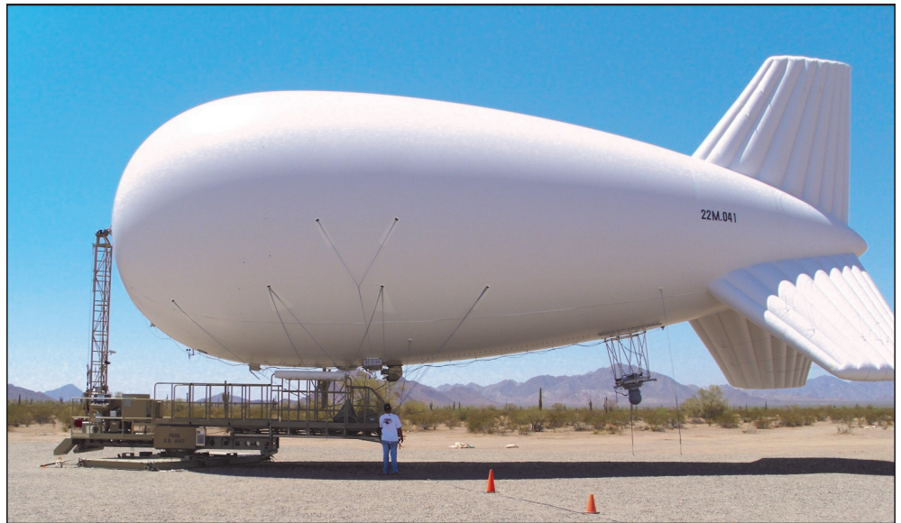
A Persistent Ground Surveillance System (PGSS) aerostat undergoes testing before deploying to an overseas combat location. The Rapid Response community within the Naval Air Warfare Center Aircraft Division created the PGSS aerostat in response to urgent and emergent warfighter needs. (U.S. Navy photo)
