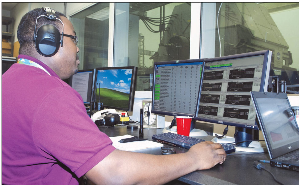
Tony Lee, an engineer with Machinery Technology Research and Development Branch at Naval Surface Warfare Center Carderock Division – Ship Systems Engineering Station (NSWCCD-SSES) monitors testing of a 7,000-rpm, 14-megawatt High Speed Generator (HSG) at the Land Based Test Site (LBTS). The prototype provides up to six times more power than lower speed, conventionally cooled, similar sized generators currently available. Photo by Martin Sheehan.
