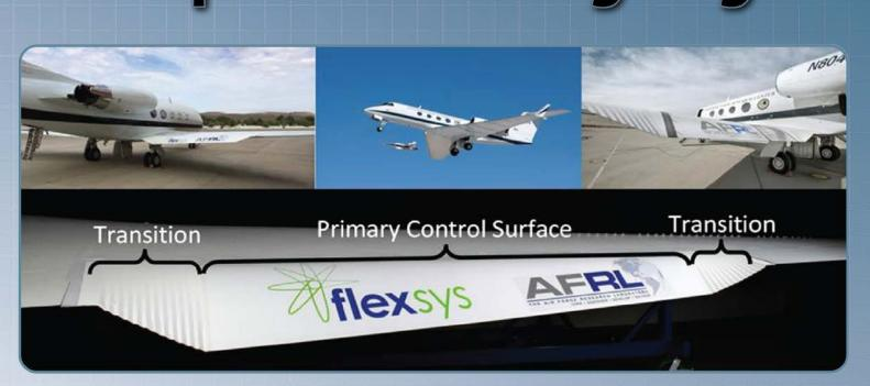
AFRL partnered with FlexSys and NASA to mature the compliant trailing edge technology. Successfully flown Adaptive Compliant Trailing Edge as part of NASA ERA in June 2015
