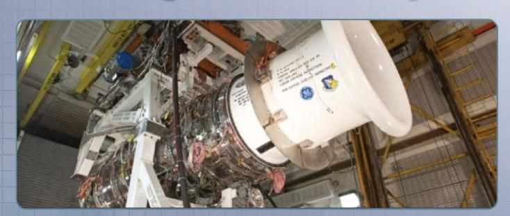
Completed 47 hours of test on an adaptive engine. Tests were done over a wide throttle range and acquired data to characterize adaptive features, validate fuel consumption, and performance
