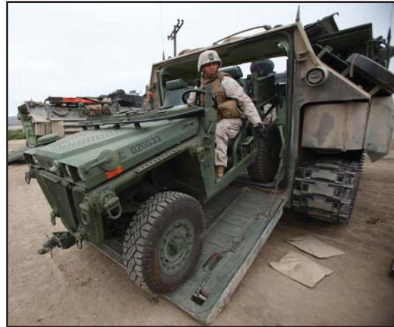
An ITV being offloaded from an AAV
