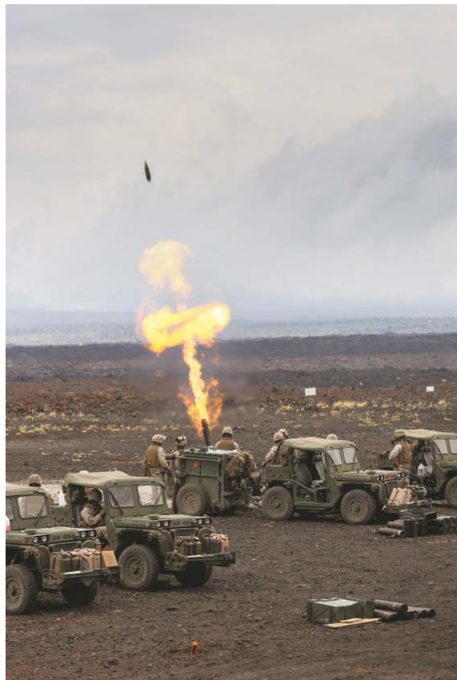
ITVs aligned and conducting a fire mission with the Expeditionary Fire Support System
