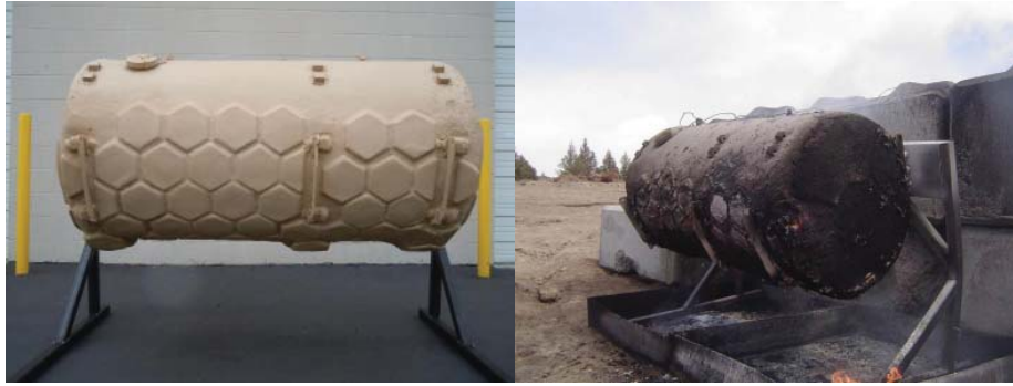
Before and after results of pool fire testing at Aberdeen Test Center. Left photo: Prepared Test Vessel; Right photo: Fuel tank with full volume of fuel post fire
