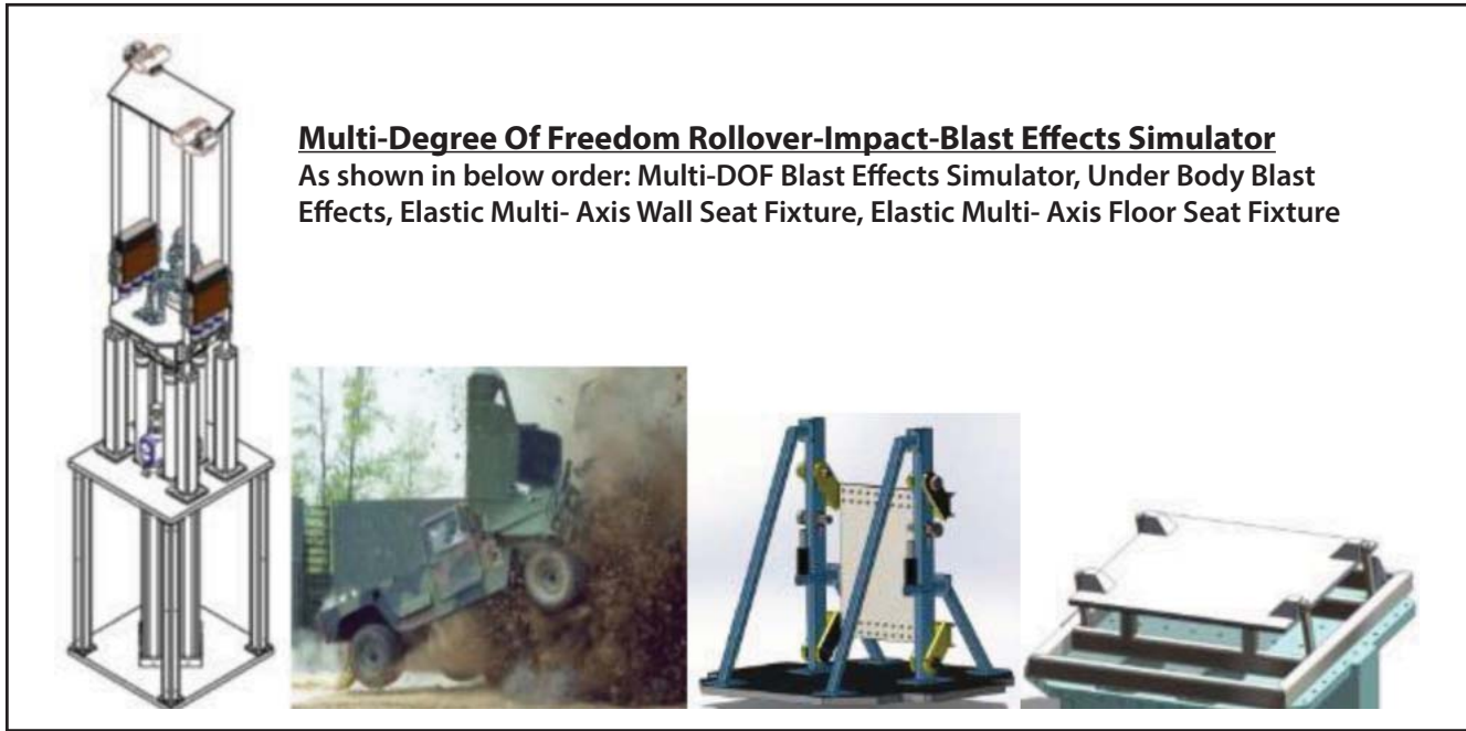
Figure 6.2-1. Multi-Degree Of Freedom Rollover-Impact-Blast Effects Simulator
