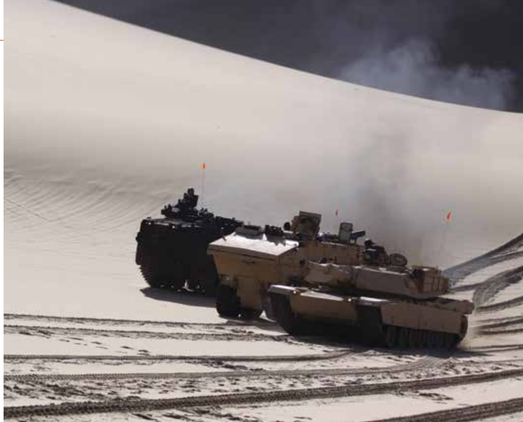
Comparative analysis of soft-soil mobility between the AAVP7, the MPC-TD, and the M1A1 Abrams tank, conducted at Sand Mountain State Park, Nev.
