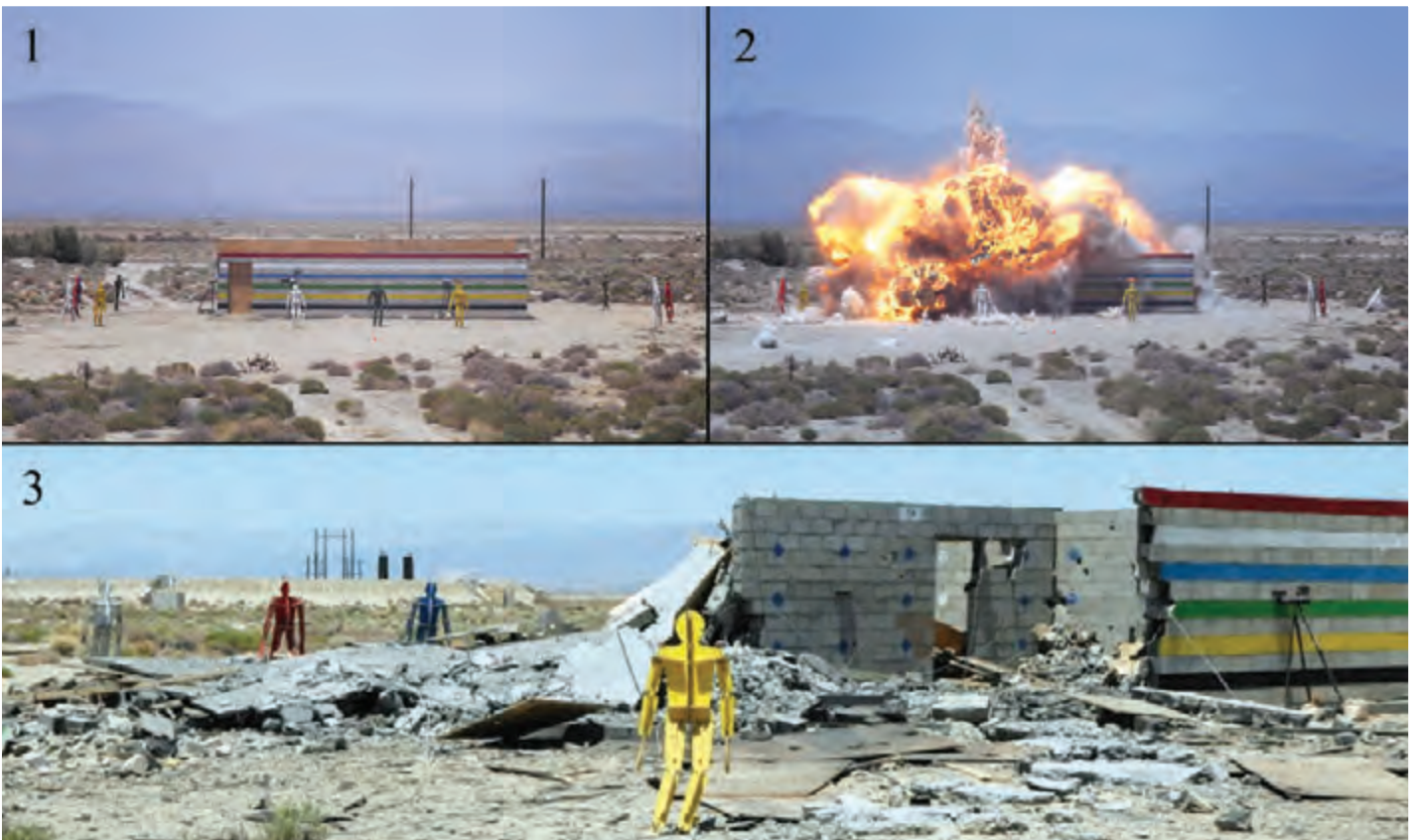
Low Collateral Damage Bomb impact test conducted at the NAVAIR Land Range, China Lake, California. (U.S. Navy Photos)
