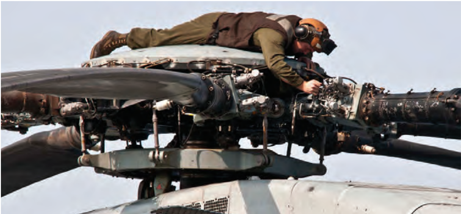
A Marine does a final check on the rotor of a CH-53E helicopter during flight operations aboard USS New York (LPD 21). (Photo by MCSN Cyrus Roson)
