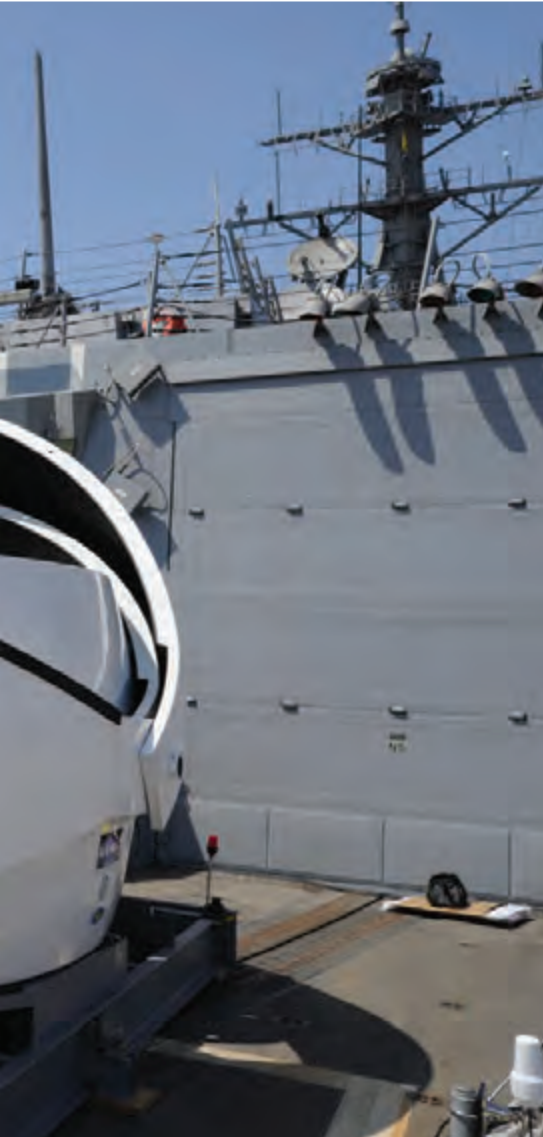
The Laser Weapon System (LaWS) temporarily installed aboard the guided-missile destroyer USS Dewey (DDG 105). The Office of Naval Research's Solid State Laser (SSL) portfolio includes LaWS development and upgrades providing a quick reaction capability for the fleet with an affordable SSL weapon prototype. (Photo by John F. Williams)
