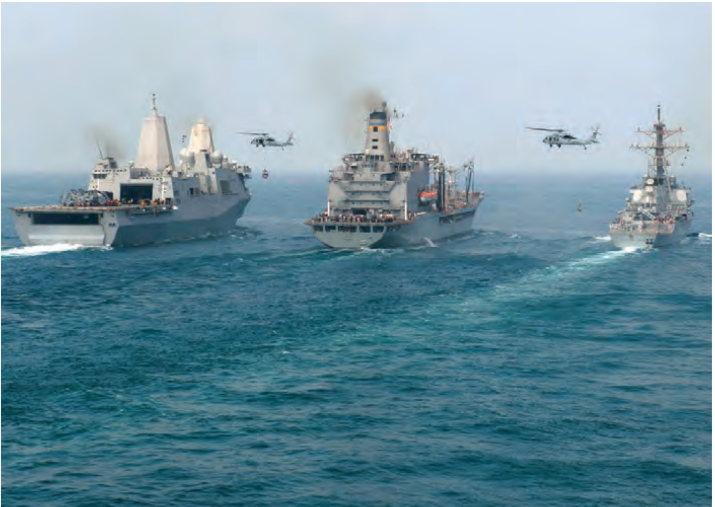
USNS Patuxent (T-AO 201), center, conducts a simultaneous replenishment at sea with the amphibious transport dock ship USS New Orleans (LPD 18), left, and USS John Paul Jones (DDG 53). (Photo by MC2 Jason Behnke)
