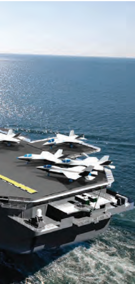
An artist's rendering of an America-class amphibious assault ship. USS Tripoli (LHA 7) will be 844 feet long, 106 feet wide and will displace 44,971 tons. (Courtesy of Huntington Ingalls Industries)
