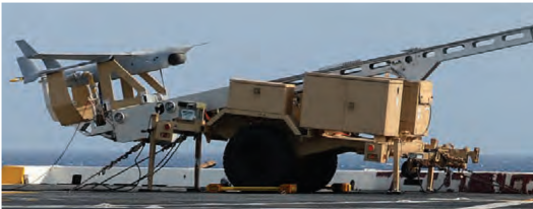
The MKIV launcher prepares to launch the RQ-21A Small Tactical Unmanned Air System (STUAS) from the flight deck of USS Mesa Verde (LPD 19) for its first flight at sea. (Photo by MC2 Stuart Phillips)
