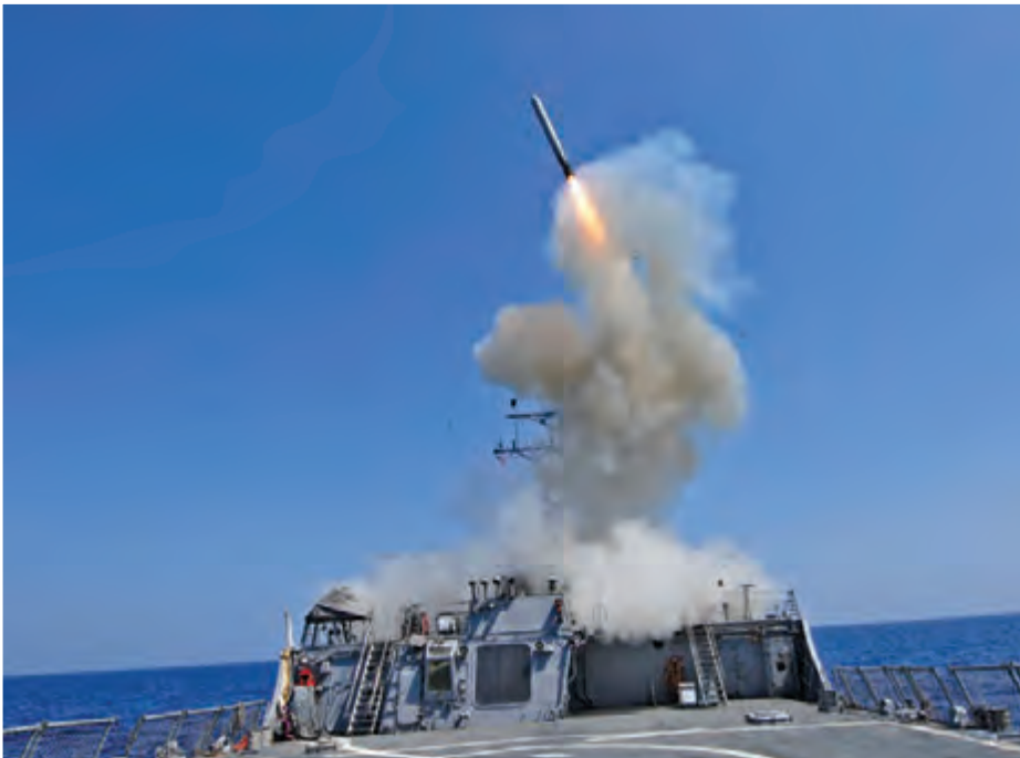
The Arleigh Burke-class guided missile destroyer USS Barry (DDG 52) launches a Tomahawk cruise missile. (Photo by MC3 Jonathan Sunderman)
