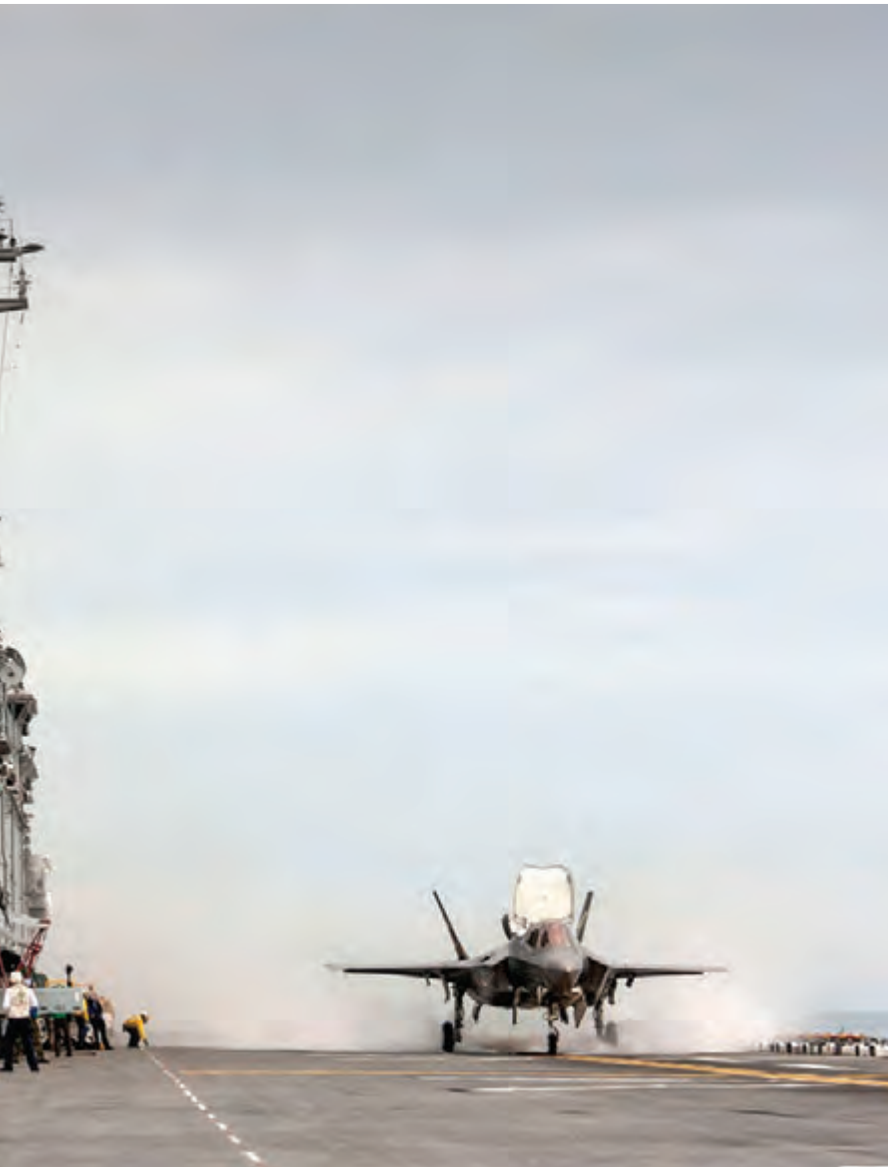
F-35B Aircraft BF-1 and BF-5 perform STOVL operations aboard the USS Wasp (LHD 1). (Photo Courtesy of Lockheed Martin)
