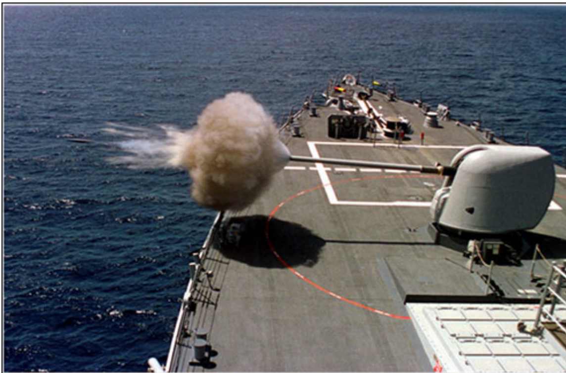
Arleigh Burke-class guided missile destroyers are equipped with a 5-inch (127-millimeter) gun.
