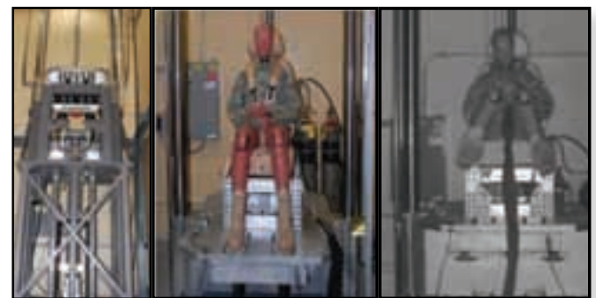
The ONR Crew Seating Blast Effects Simulator is used to simulate vehicle blast effects accelerations to validate crew-seat protection concept models and devices.
