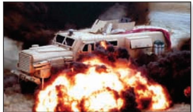
A MRAP undergoes testing at Aberdeen Test Center, Md.
