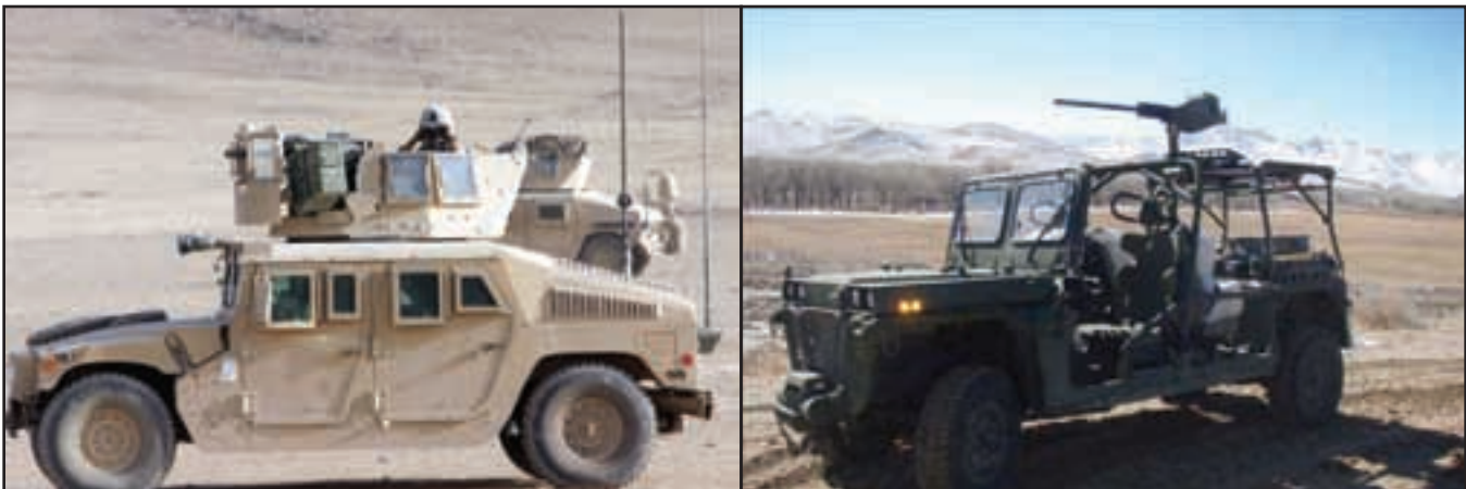
Left Photo: The weight of the up-armored HMMWV had resulted in maintenance and logistic issues. Right Photo: Contrasting HMMWV, the ITV is light weight and highly transportable.
