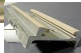
Improved coating on missile rail surfaces: 10x improved wear
