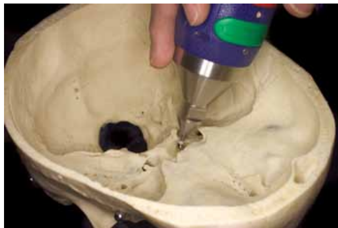
3 Measurement of sella turcica, fiducial marker position on control using 3 mm contact probe.
