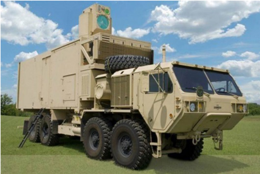
A 10-kilowatt laser weapon is mounted on a High-Energy Laser Mobility Tactical Truck. (Courtesy photo/U.S. Army Space and Missile Defense Command)
