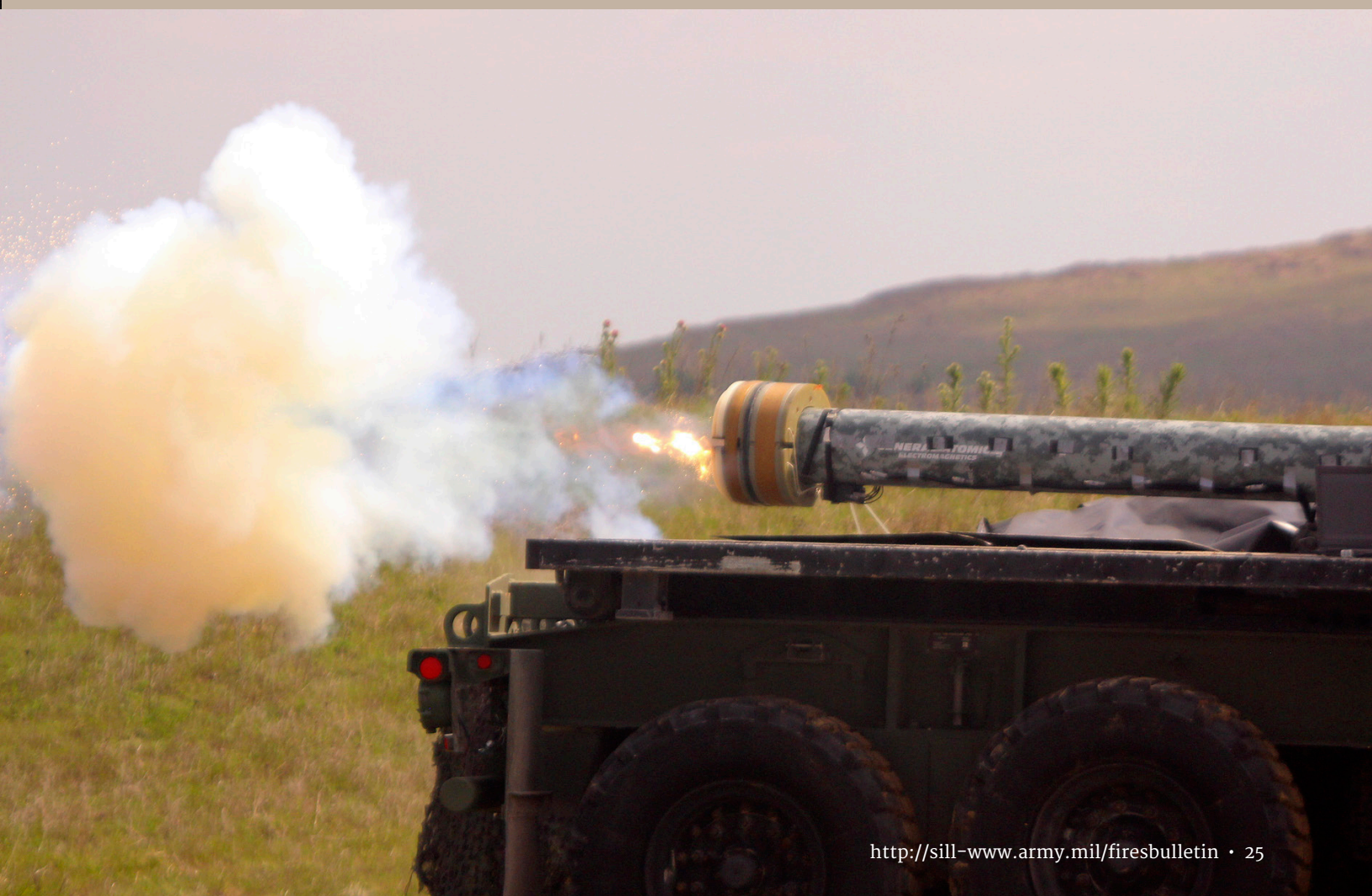
A projectile, traveling at six times the speed of sound, leaves the muzzle of a railgun April 19 on a Fort Sill training area during the Maneuver Fires Integration Experiment 2016. (Monica Wood)
