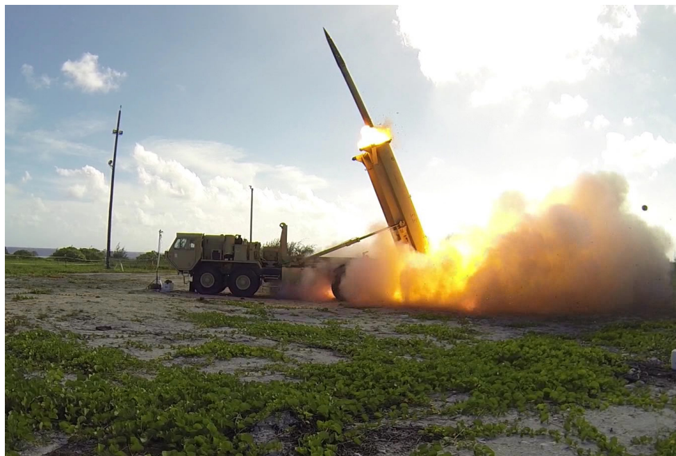
A Terminal High Altitude Area Defense (THAAD) interceptor is launched from a THAAD battery located on Wake Island, during Flight Test Operational-02 Event 2a. During the test, the THAAD system successfully intercepted two air-launched ballistic missile targets. (U.S. Missile Defense Agency)
