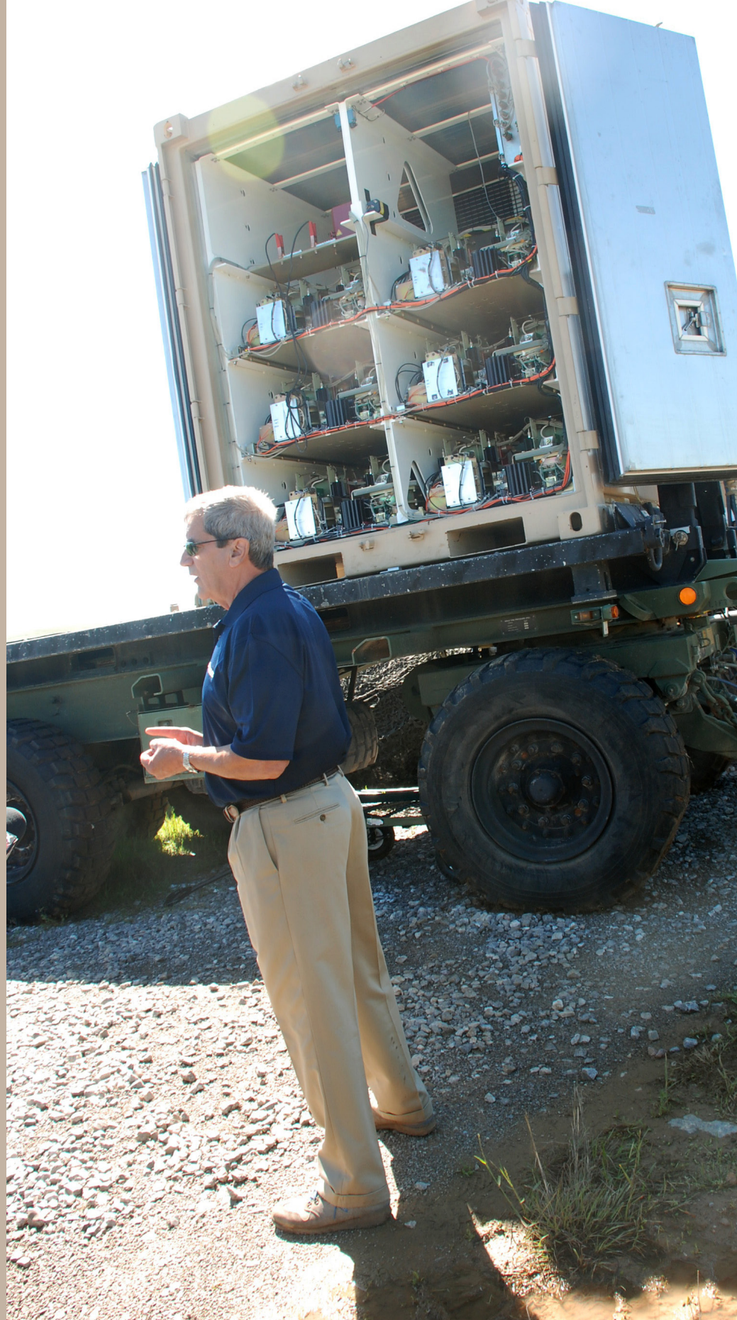
Robert Taylor, who was involved with the payload and design at General Atomics, explains how the power system is set up in a modular format, meaning if one is lost, the others can be manipulated to pick up the slack, during the Maneuver Fires Integrated Experiment, at Fort Sill, Okla., April 21. (Monica Gutherie/Fort Sill Tribune)
