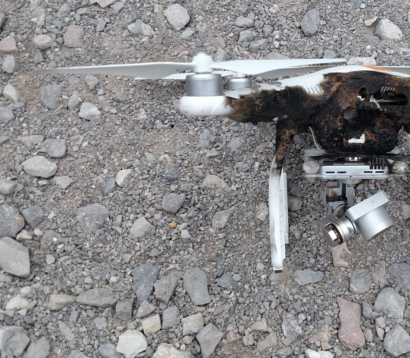
A 5-kilowatt laser weapon system damages an the unmanned aerial system. (Capt. Jeff Jaramillo/U.S. Army)
