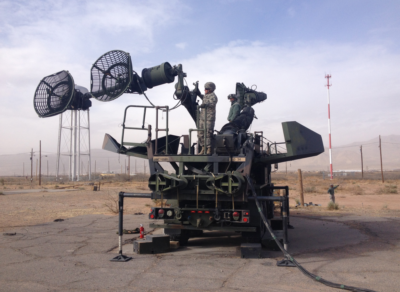
PFC James Barkley and SPC Kevin Olivier emplace the Patriot Antenna Mast Group during march-order and emplacement training in Tobin Wells, Fort Bliss, Texas. (Photo courtesy of CPT Joshua A. Urness)
