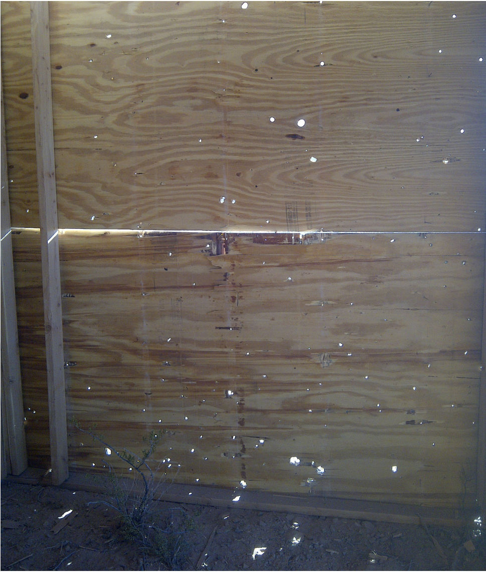
Damage sustained to the target post-impact. (Photo courtesy of LTC Gary C. Leroux)
