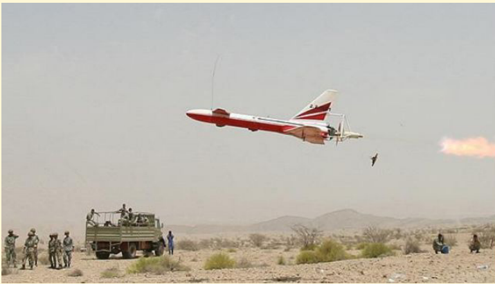
Iranian Ababil UAS conducting a launcher supported take-off for testing operations. (Photo courtesy of By MAJ (Ret.) F. Patrick Filbert and USAF Maj. (Ret.) Darryl Johnson)
