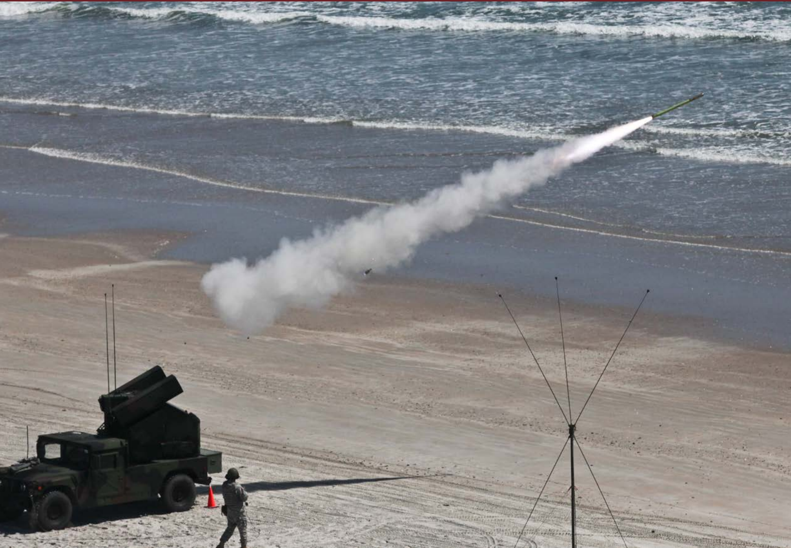
A Stinger missile is fired from the Avenger weapon system at an aerial target off the coast on Onslow Beach, Camp Lejeune, N.C., March 15, 2013. The target scale is one-fifth the size of an actual aircraft, giving units a realistic target with which to train. The training allowed the 2nd Battalion, 263rd Air Defense Artillery to set up in a deployment formation versus the usual static formation at other smaller training sites. (Photo by Cpl. Austin Long, U.S. Marine Corps)
