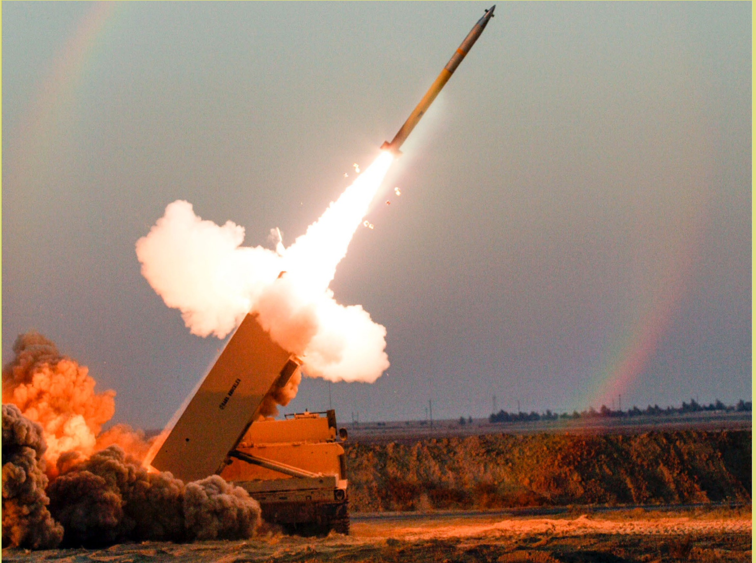
A Guided Multiple Launch Rocket System (GMLRS) from A Battery, 2nd Battalion, 4th Field Artillery, fires a 227 mm rocket. (Photo by Rick Rzepka, U.S. Army)
