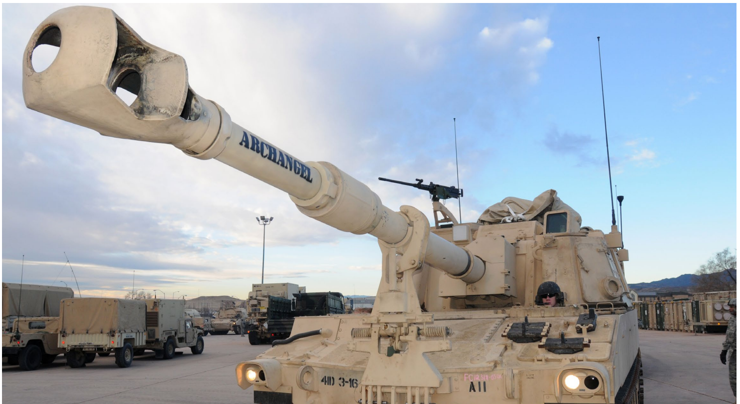
SPC Rodney Nichols, cannon crew member, A Battery, 3rd Battalion, 16th Field Artillery, 2nd Brigade Combat Team, 4th Infantry Division, positions an M109A6 Paladin self-propelled howitzer in preparation to conduct a field exercise on Fort Carson, Colo. (Photo by SSG Andrew Porch, U.S. Army)
