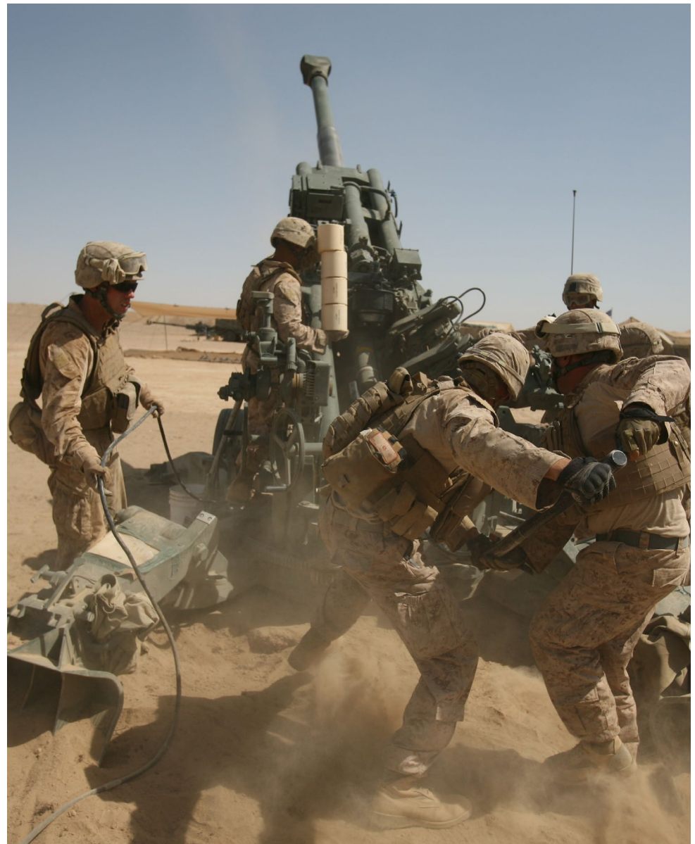
Marines from Gun-3, A Battery, 1st Battalion, 12th Marines, ram a satellite-guided Excalibur XM982 Precision Engagement Projectile during a fire mission on Fire Base Saenz, Helmand province, Afghanistan. (Photo by SGT Earnest J. Barnes, U.S. Army)
