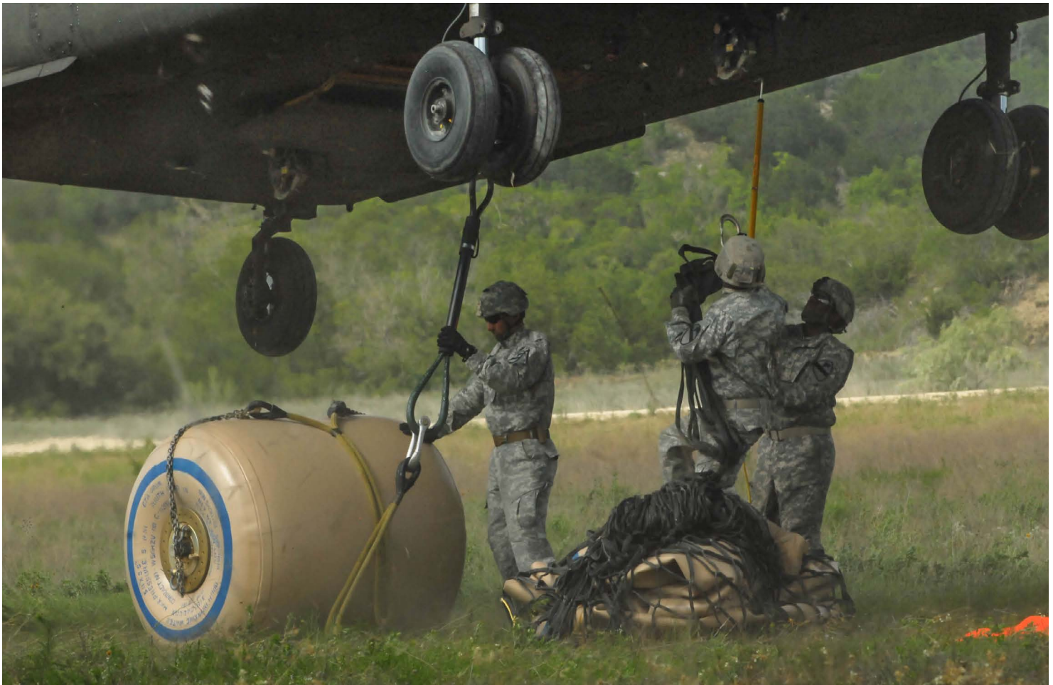
SPC Palo Gonzalez, a petroleum supply specialist (left), SGT Billy Taylor a motor transport operator (center) and SSG Eric Barnett also a petroleum supply specialist, all assigned to Company A, 115th, Muleskinner , Brigade Support Battalion, 1st Ironhorse Brigade Combat Team, 1st Cavalry Division, attach a water blivet and cargo net to a CH-47 Chinook helicopter while conducting sling load training during the Brigade Support Area exercise June 1, at Fort Hood, Texas. (Photo by SSG John Couffer, 1st BCT Public Affairs, 1st CAV)
