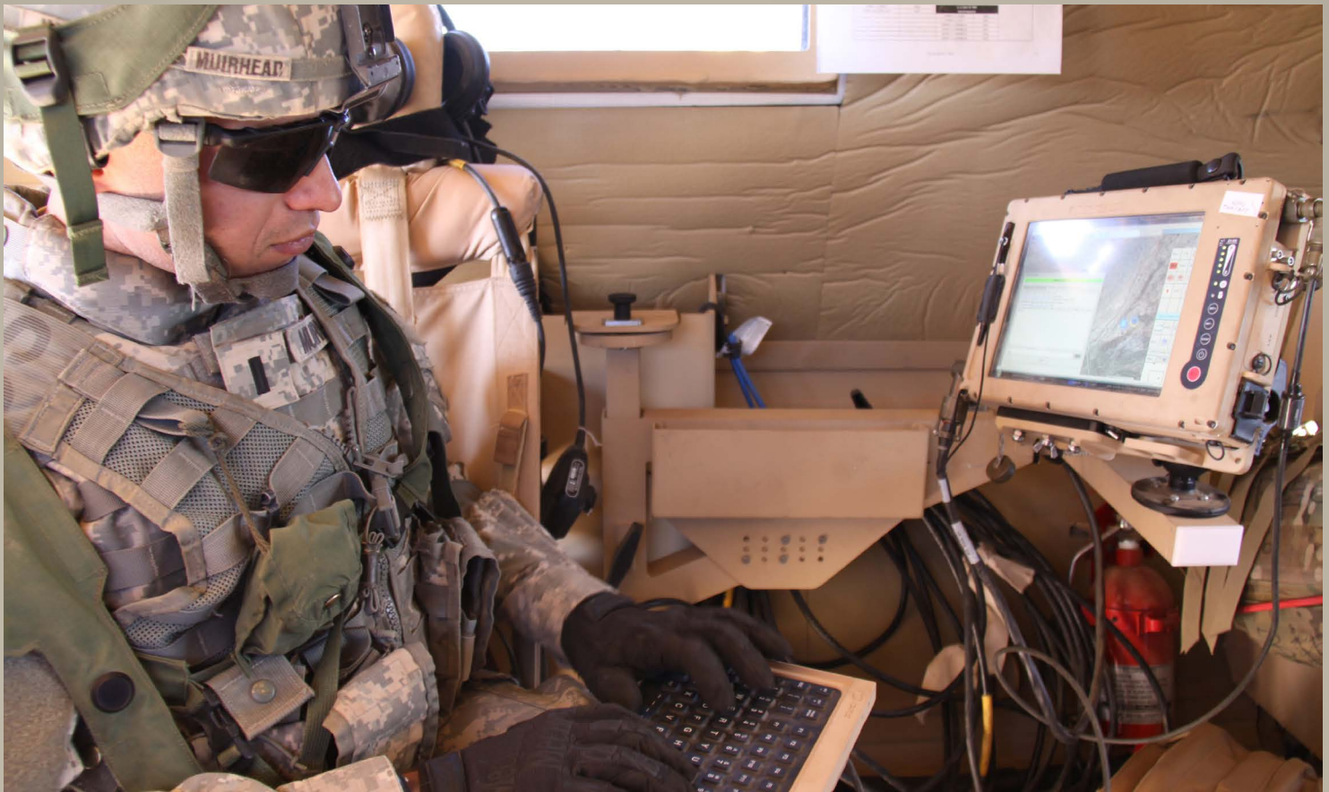
A 2nd Brigade, 1st Armored Division Soldier uses the new chat feature of the Joint Capabilities Release of Force XXI Battle Command Brigade and Below/Blue Force Tracking during NIE 12.1 in November. Joint Capabilities Release Chat works like an online chat room within FBCB2, allowing users to instant-message in real time over the BFT 2 satellite network. Joint Capabilities Release is part of Capability Set 13. (Photo by Claire Schwerin; U.S. Army)
