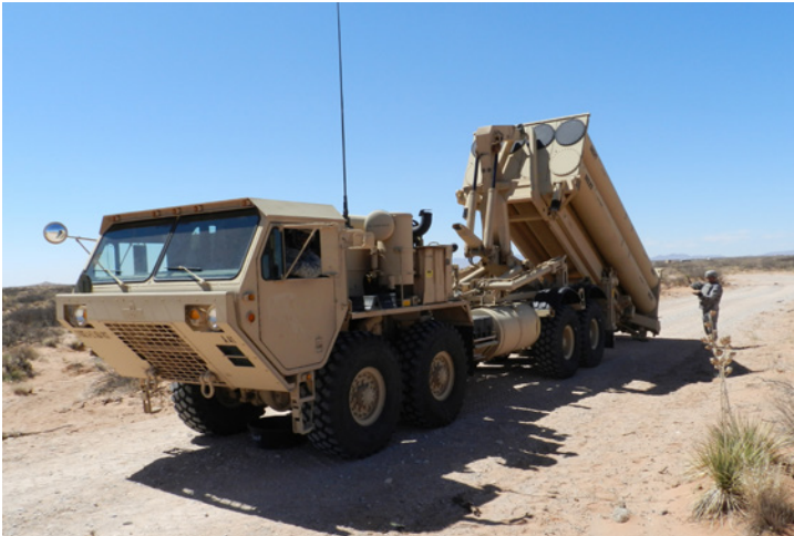
A Soldier with A Battery, 2nd Air Defense Artillery, Terminal High Altitude Area Defense (THAAD), helps ground guide a vehicle during emplacement of a missile launcher. (Photo courtesy of 11th Air Defense Artillery Brigade)
