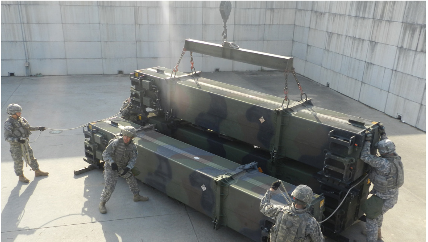
Launcher crew members from the 94th Army Air and Missile Defense Command work together to lower and align the simulated spent missile canisters during reload training. (Photo by SPC Issac Castleberry, U.S. Army)
