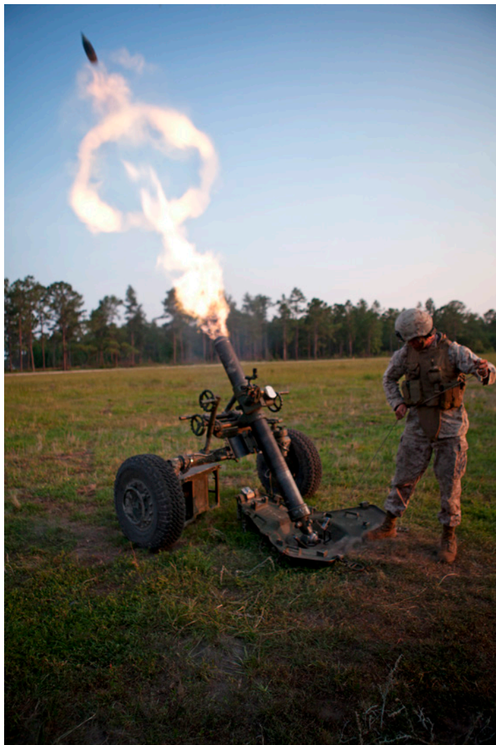
A Marine from 10th Marine Regiment fires a 120 mm towed rifled mortar system, known as the Expeditionary Fire Support System. (Photo courtesy of 10th Marine Regiment)
