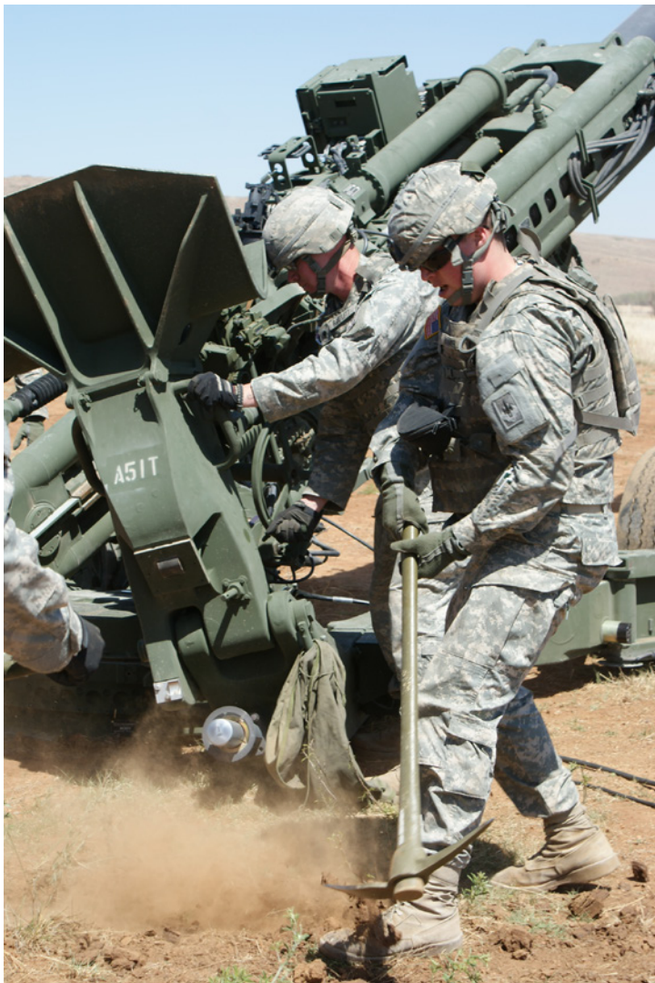
Soldiers from A Battery, 1st Battalion, 129th Field Artillery digging in the M777A2's spade. (Photo courtesy of 1st BN, 129th FA)
