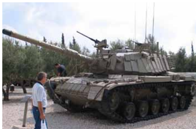
(Left) Figure 1. How an ERA works. (Above) Figure 2. M60 Patton Tank Fitted with ERA Plates (Information and figure provided by Howard Kleinberg)
