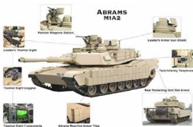
Figure 3. U.S. Army M1A2 tank urban survival kit (TUSK) system enhancement package (SEP), which includes, among many other upgrades, ERA plates attached to the tank's side-skirts to protect the tank from being disabled by anti-tank Fires. (Information and figure provided by Howard Kleinberg)
