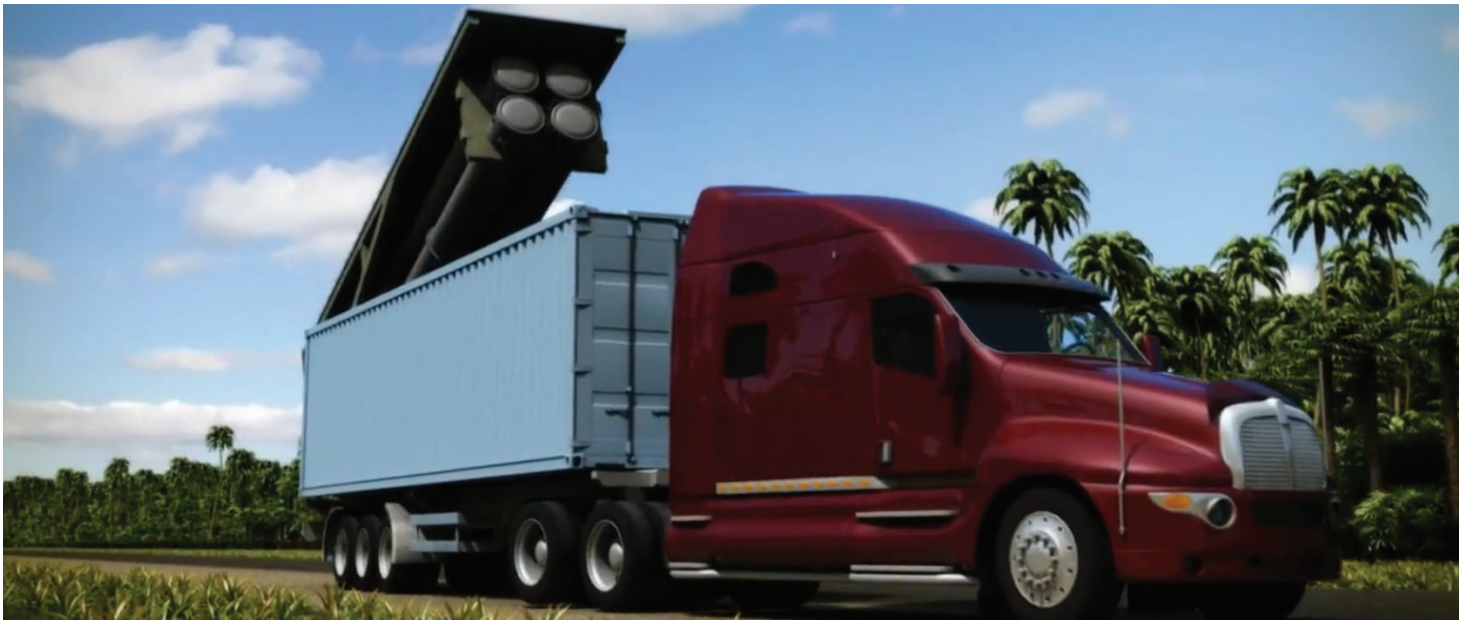
The Club-K Missile System is being transported by land using a semi-truck, while hidden inside an ISO cargo container. (Photo illustration courtesy of ConcernAgat)
