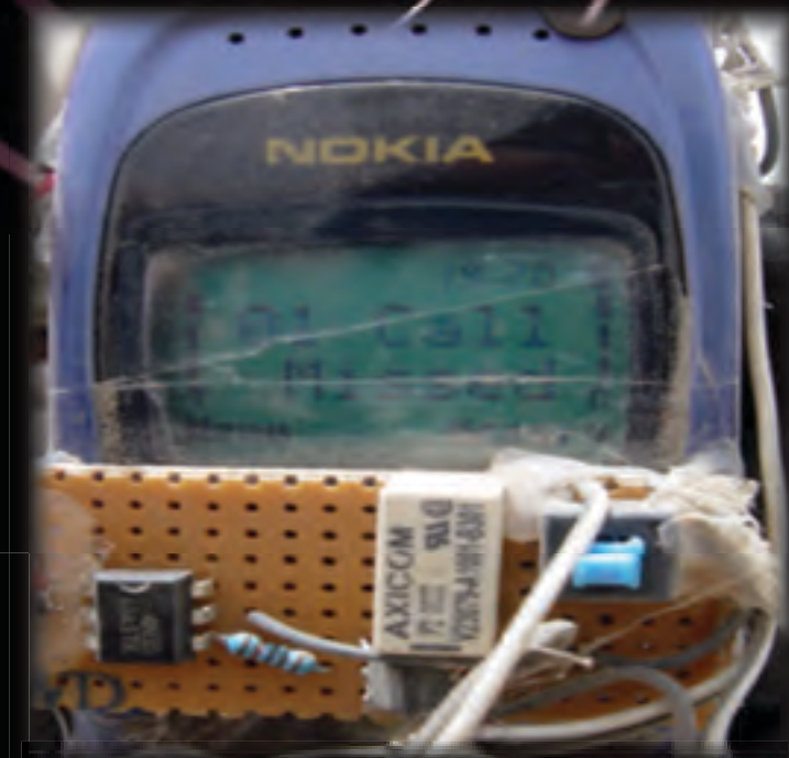
This cell phone was rigged as a detonator for an improvised explosive device. The detonator was recovered undamaged after having been successfully jammed by electronic warfare personnel using Counter Radio-Controlled IED Electronic Warfare equipment funded by the Joint Improvised Explosive Device Defeat Organization. (Photo courtesy of the Department of Defense)
