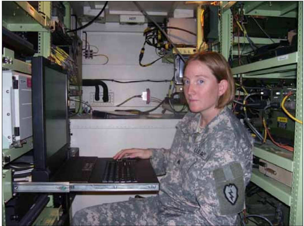
ADAM cell specialist SGT Annia Rowe of 3rd Brigade Combat Team, 25th Infantry Division, confirms connectivity on the Tactical Airspace Integration System Bullfrog computer system inside the Air Defense and Airspace Management Shelter in Tikrit, Iraq, Oct. 5, 2007. The ADAM shelter is organic equipment to all brigade aviation elements in infantry brigade combat teams and contains a full suite of communications and airspace management systems. (Photo courtesy of 25th Combat Aviation Brigade Public Affairs)
