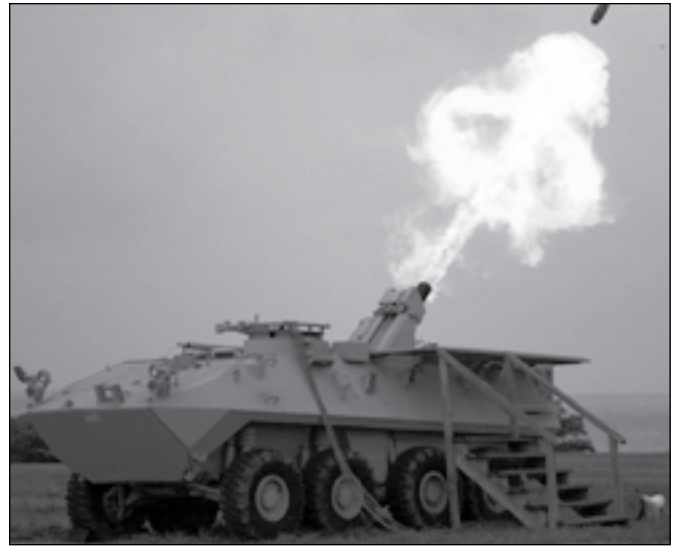
The XM-326 Dragon Fire II in its light armored vehicle configuration during firing tests at the Naval Surface Weapons Center Dahlgren, Dahlgren, Va. in 2004. (Photo courtesy of LtCol. [Retired] Forrest R. Lindsey)
