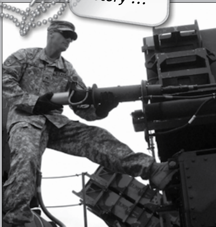
SGT Bryan E. Toler helps crew members install an antenna on a Patriot launcher station during march order and emplacement. (Photo by SGT Valenzuela, U.S. Army)
