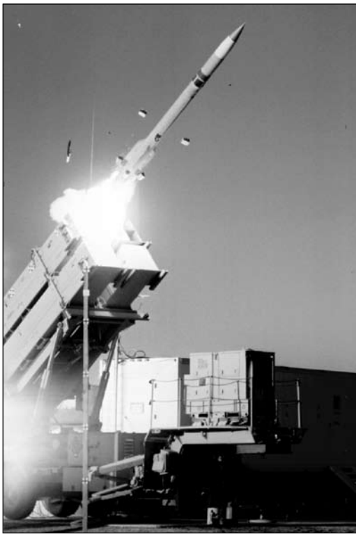
A Patriot Advanced Capabilities (PAC)-3 launches during testing at White Sands Missile Range in New Mexico. Patriot is a high- to medium-altitude air defense system designed to intercept tactical ballistic missiles (TBMs) and “air-breathing” threats. (Photo courtesy of Lockheed Martin)
