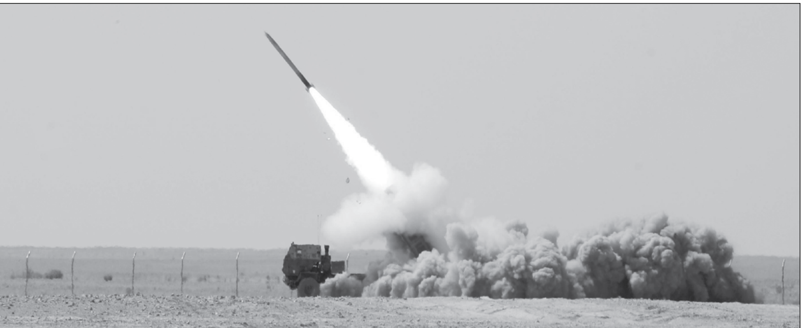
The US Marines fire the GMLRS Unitary from their High-Mobility Artillery Rocket System (HIMARS) in Iraq.
